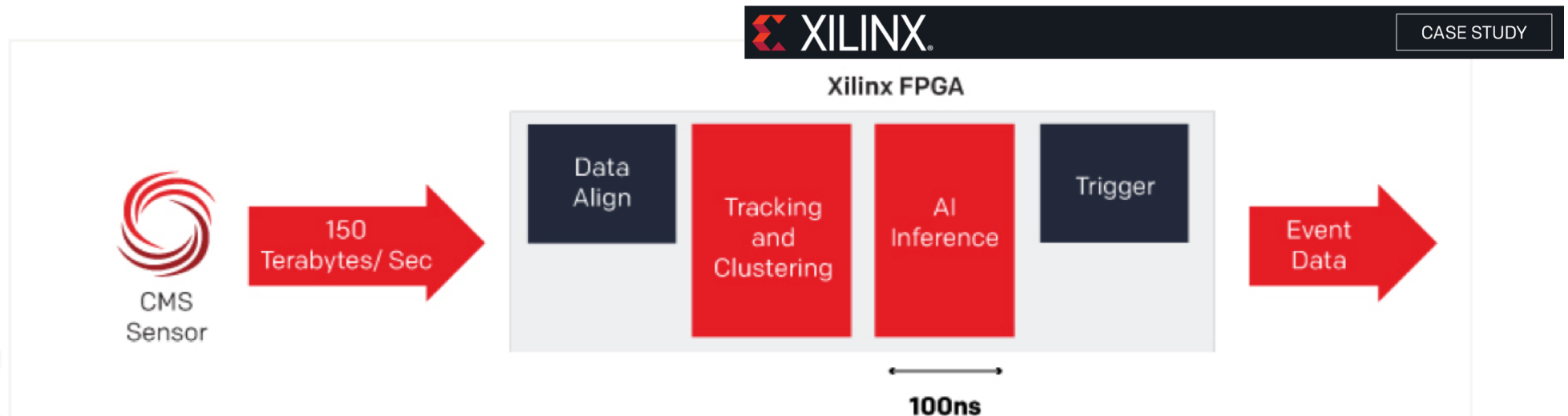
Figure 2: Compared to alternative devices such as GPUs and ASICs, FPGAs are the only viable choice for the event trigger processing because they provide extremely low latency. While the large numerical processing capability of GPUs is attractive, these technologies are optimized for high throughput, not low latency.
