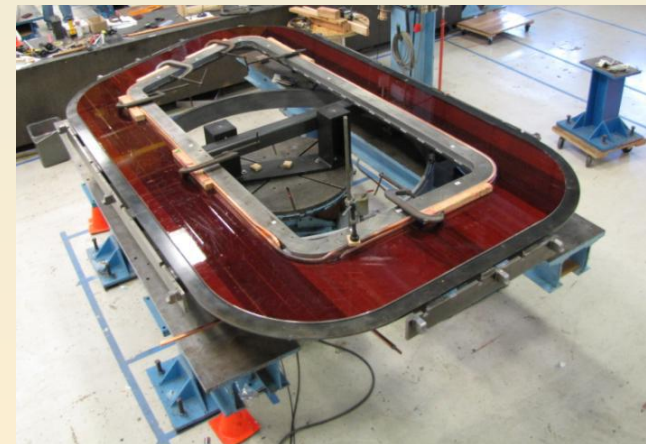
CLAS12 Torus coil winding table at FNAL
