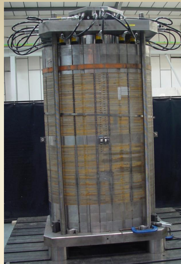
Q1 Magnet Yoke Stack complete at SMI, UK
