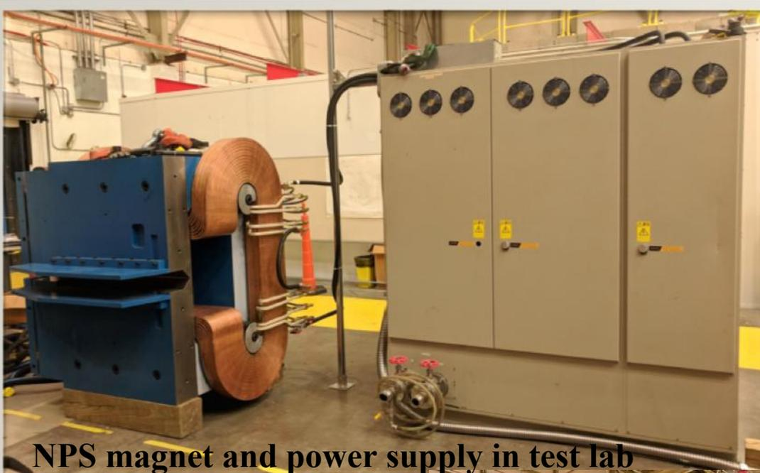
NPS magnet and power supply in test lab
