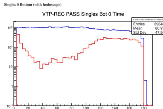
Effect of the high hit rates on the FADC on the trigger logic (pile up hits are missed by trigger when within 32ns of each other) ~1% loss effect (roughly consistent with the FADC hit rate seen from hodoscope).
