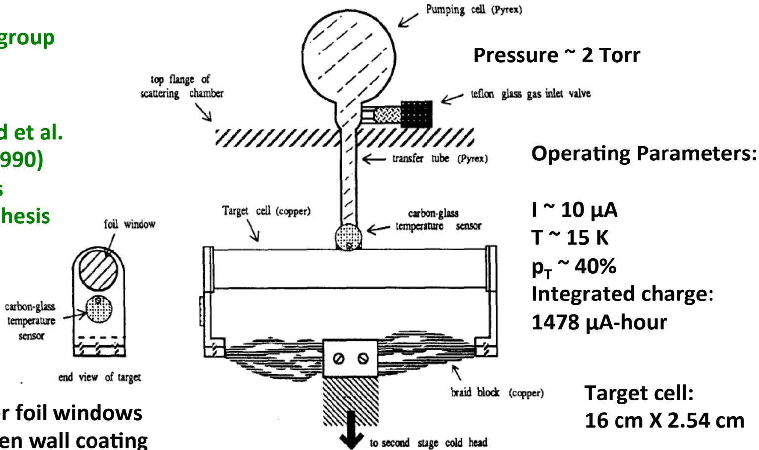
Figure 4.9: Schematic of the polarized  $^3\text{He}$  target double-cell system. The relative positions of the pumping cell, transfer tube, and target cell are shown, in addition to the braided block, the temperature sensors, and the gas inlet valve.
