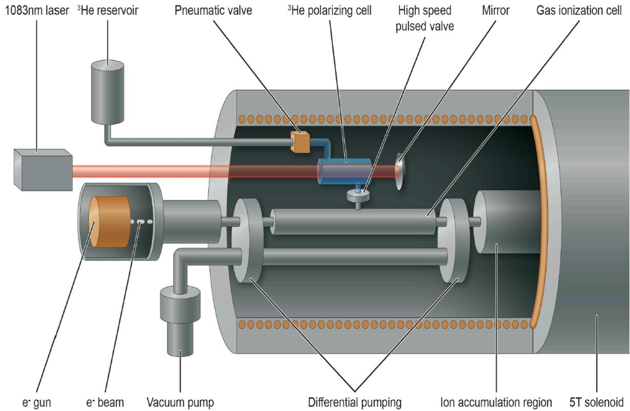
FIG. 5. Schematic layout of polarized  $^3\text{He}$  ion source under development by a BNL-MIT collaboration using optically pumped polarized  $^3\text{He}$  atoms directed into the existing Electron Beam Ionization Source.
