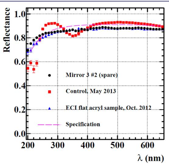
Each mirror was tested for the reflectance in both UV and Visible spectrums and 12 best mirrors for each facet were chosen.
