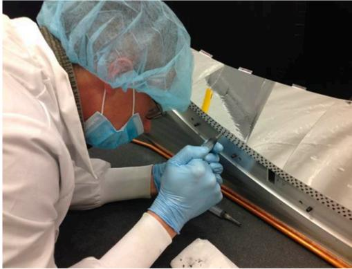
Epoxy dots were applied to one side of the mirror half sectors in the specific pattern.
