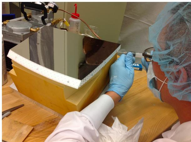
Each mirror was glued with epoxy glue using the special glue dot pattern to prevent mirror shrinkage while assuring the glue strength.
