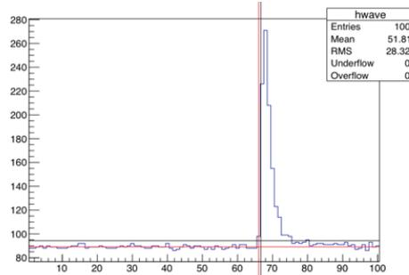
FADC spectrum in time (read from 3 ADC cards, total of 48 channels)
