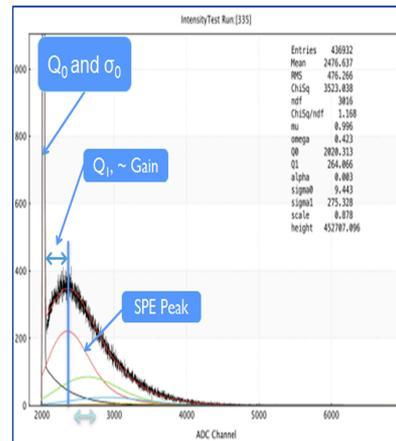
For each PMT, plot a SPE position vs High Voltage value
