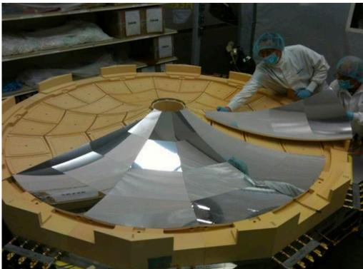
Individual half sectors were glued together on the special mirror assembly tool where they are held in place by a low pressure.
