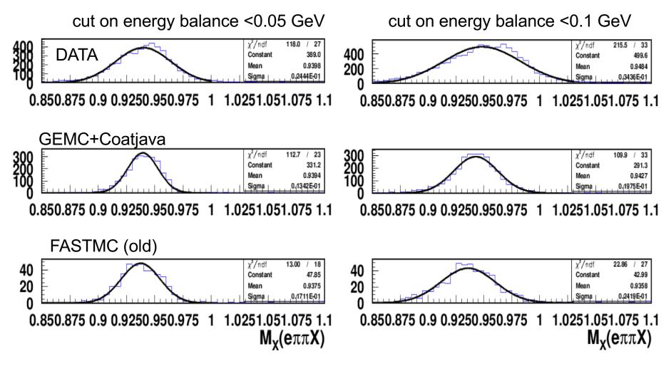
Resolution of FASTMC (specifications) missing mass is worse than gemc and better than in data (~30%)
