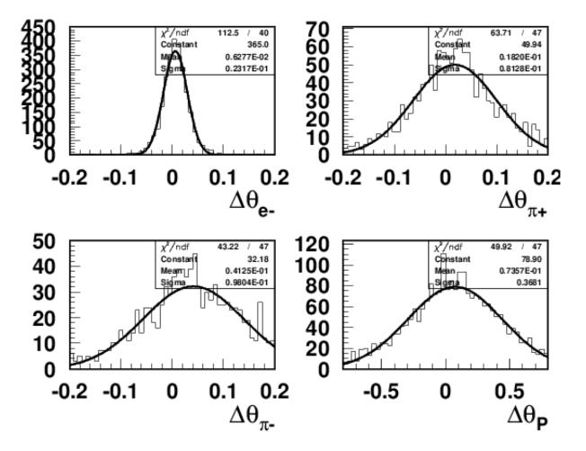
Using correct settings for reconstruction the shifts in angles are below 0.1 degree
