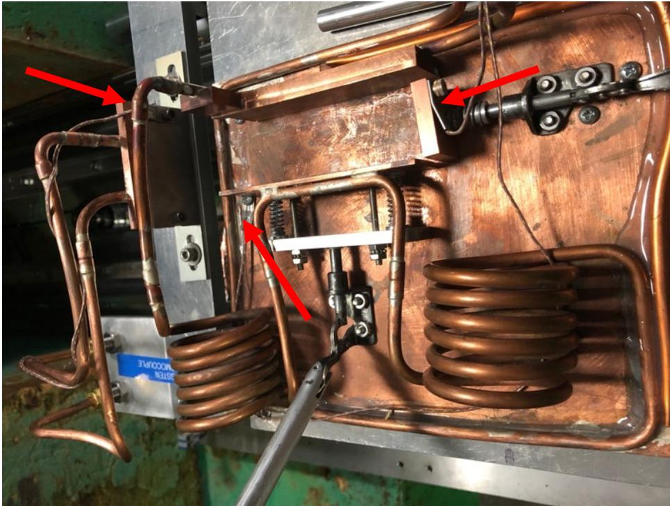
**Figure 2.** Additional TCs on the Isotope assembly
