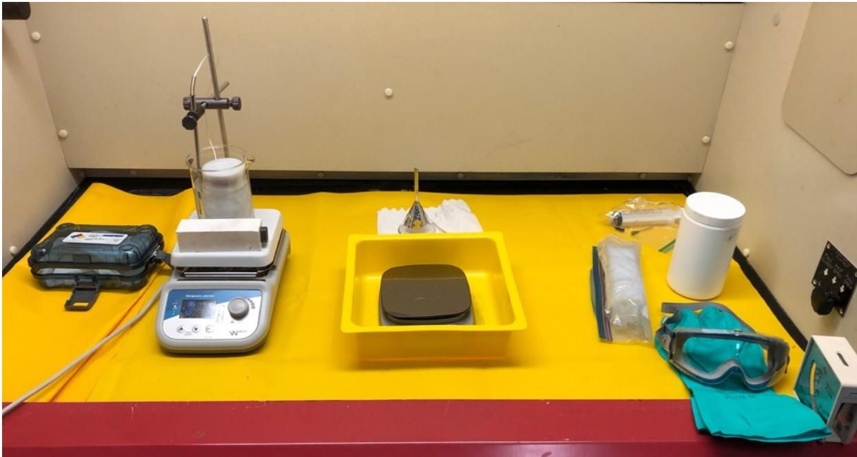
**Figure 1.** Crucible and Gallium on hot plate
