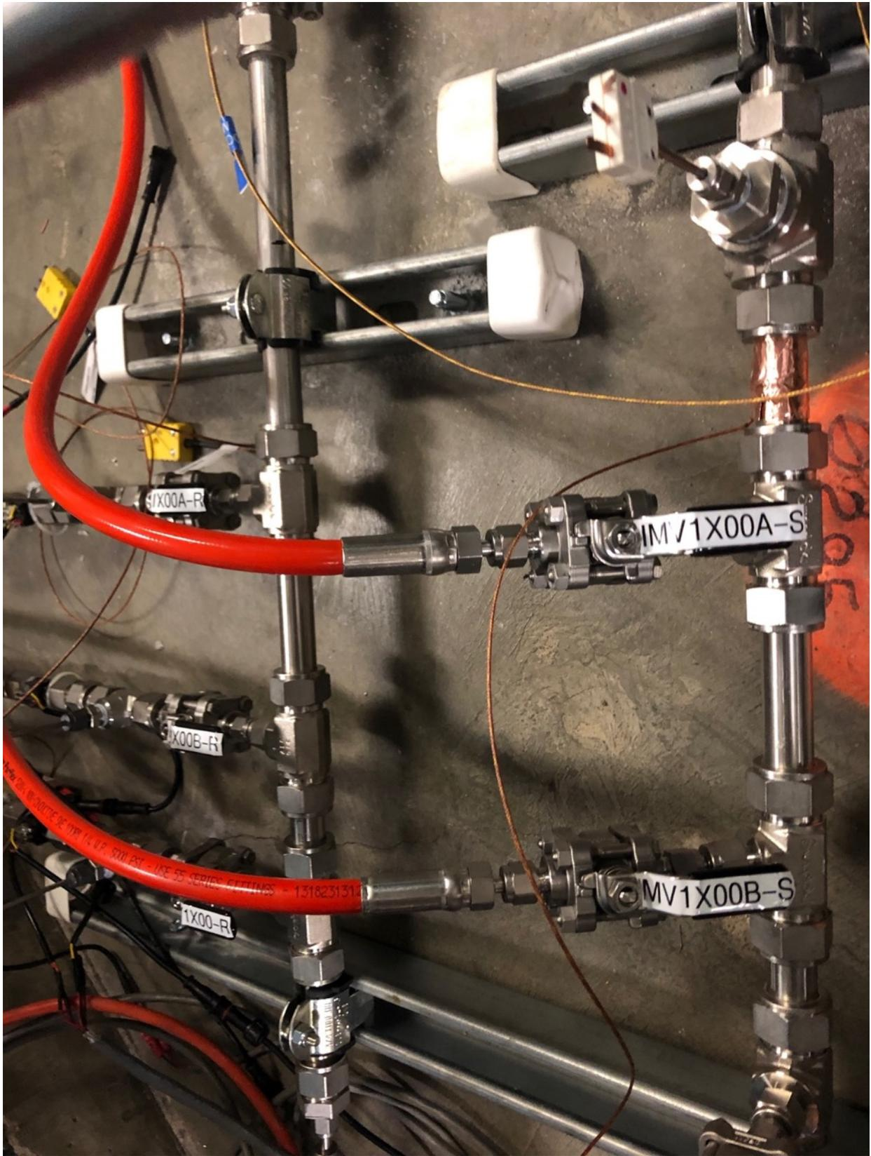
**Figure 11.** Three branch cooling circuits
