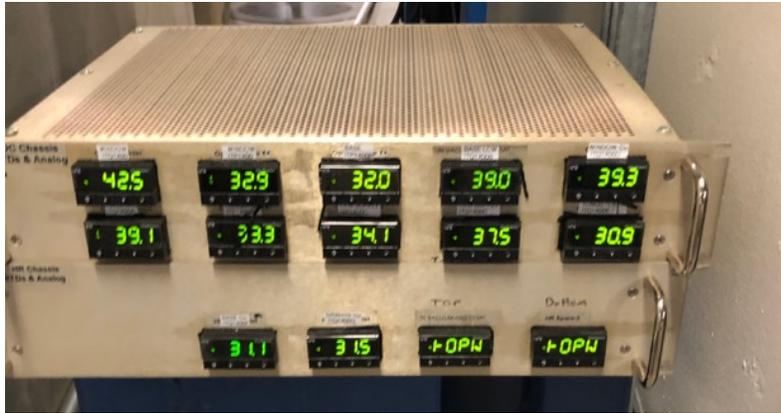
Figure 3. Omega controllers for reading out thermocouples and RTDs, 12 channels
