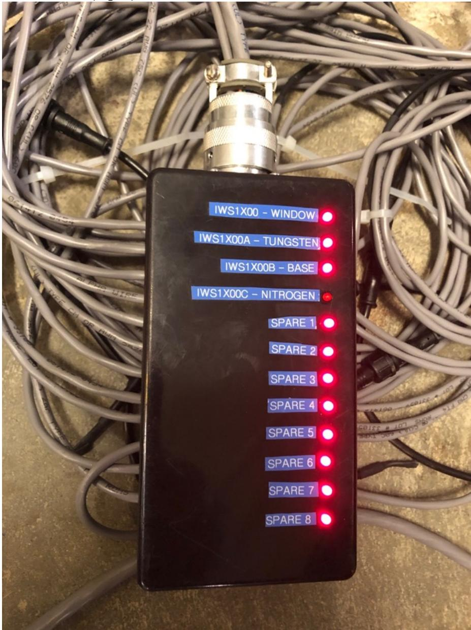
**Figure 9.** MPS Interface box. The nitrogen flow is not turned on, so the LED is off for that channel.
