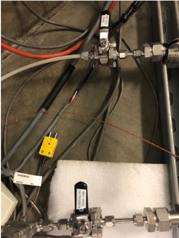
**Figure 13.** Nitrogen supply to blow circuits dry
