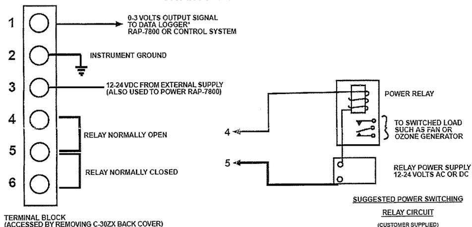
The C-30ZX internal relay is a low power device. It will handle up to 30 volts AC or DC at up to 1 amp so it will switch low voltage alarms directly. For switching power loads an intermediate relay and power supply should be used such as shown above.
