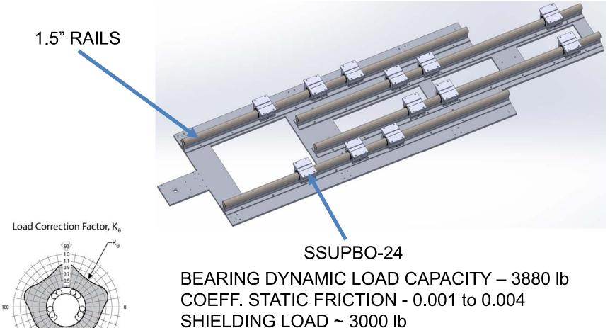
The actual dynamic load capacity of a Ball Bushing Bearing is determined by the direction of the applied load relative to the bearing circuits. The load correction factor  $K_{ij}$  is found by referring to the polar graph. To determine the actual dynamic load capacity, multiply the proper correction factor ( $K_{ij}$ ) by the dynamic load capacity. FORCE TO MOVE SHIELDING (0.004) ~ 12 lb
