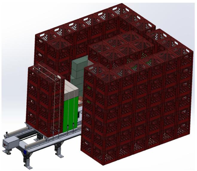
USED (10) S4 SHIELDING BLOCKS, STEEL PLATES, CONCRETE BLOCKS AND WATER FILLED MILK CRATES TO CREATE ≥13" OF STEEL AND 12" OF WATER.
