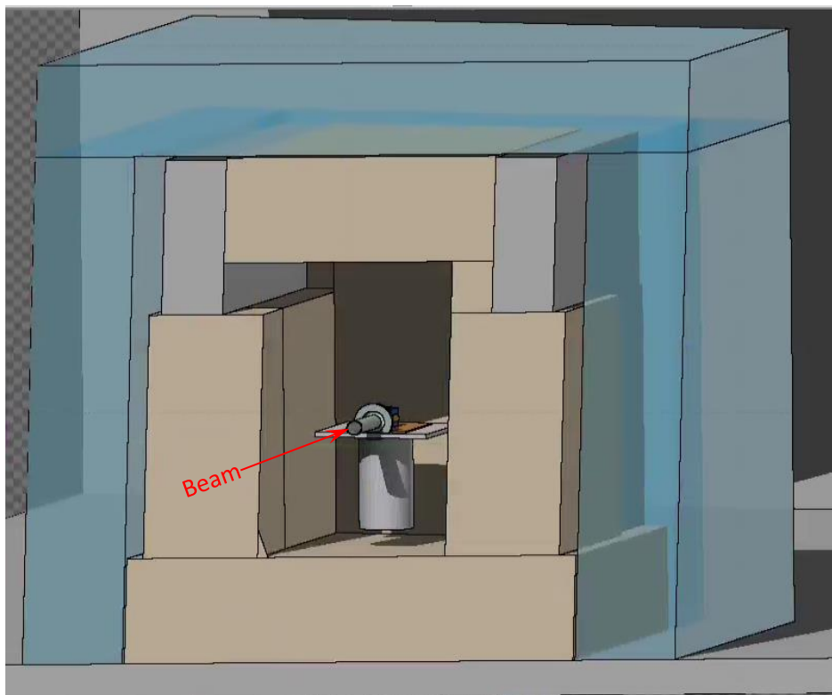
Figure 3: Cutaway of geometry for irradiation of the target within the hutch
