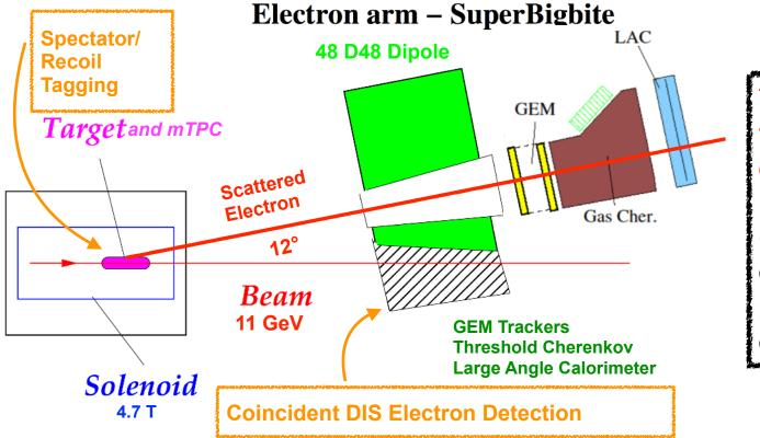
TDIS measurements very challenging: lots of exciting activities/ R&D on-going (detector simulations, design, testing, prototyping, software development)
