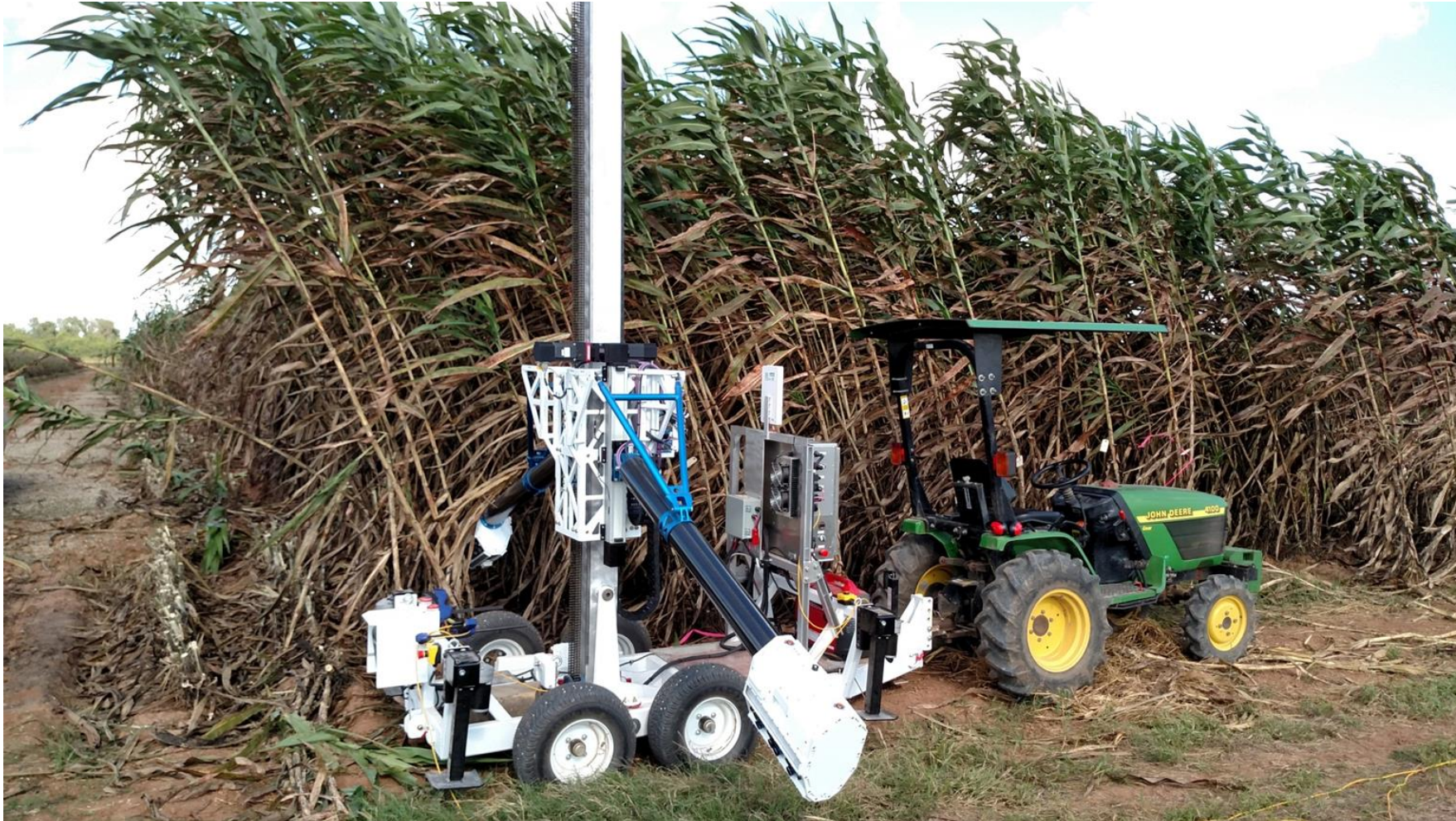
The surrogate system collecting data at the TAMU field site. The carriage supports two boom assemblies each one of which carries a sensor pod. The carriage slides up and down on the column allowing full scanning of a plant.
