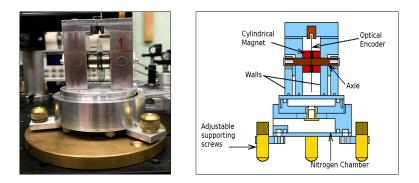
Measures the angle made by the vertical magnetic field with respect to the horizontal plane in Hall C.
