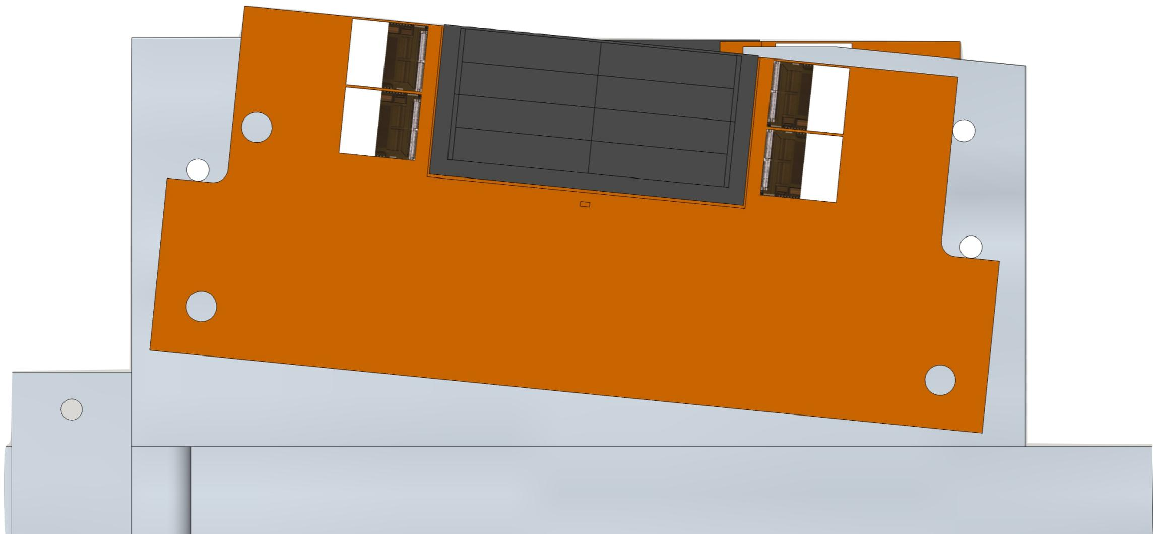
Angular acceptance of cooling block begins at 300 mrad, outside of SVT acceptance and where rate of brems is suppressed by  $>6$  orders of magnitude.
