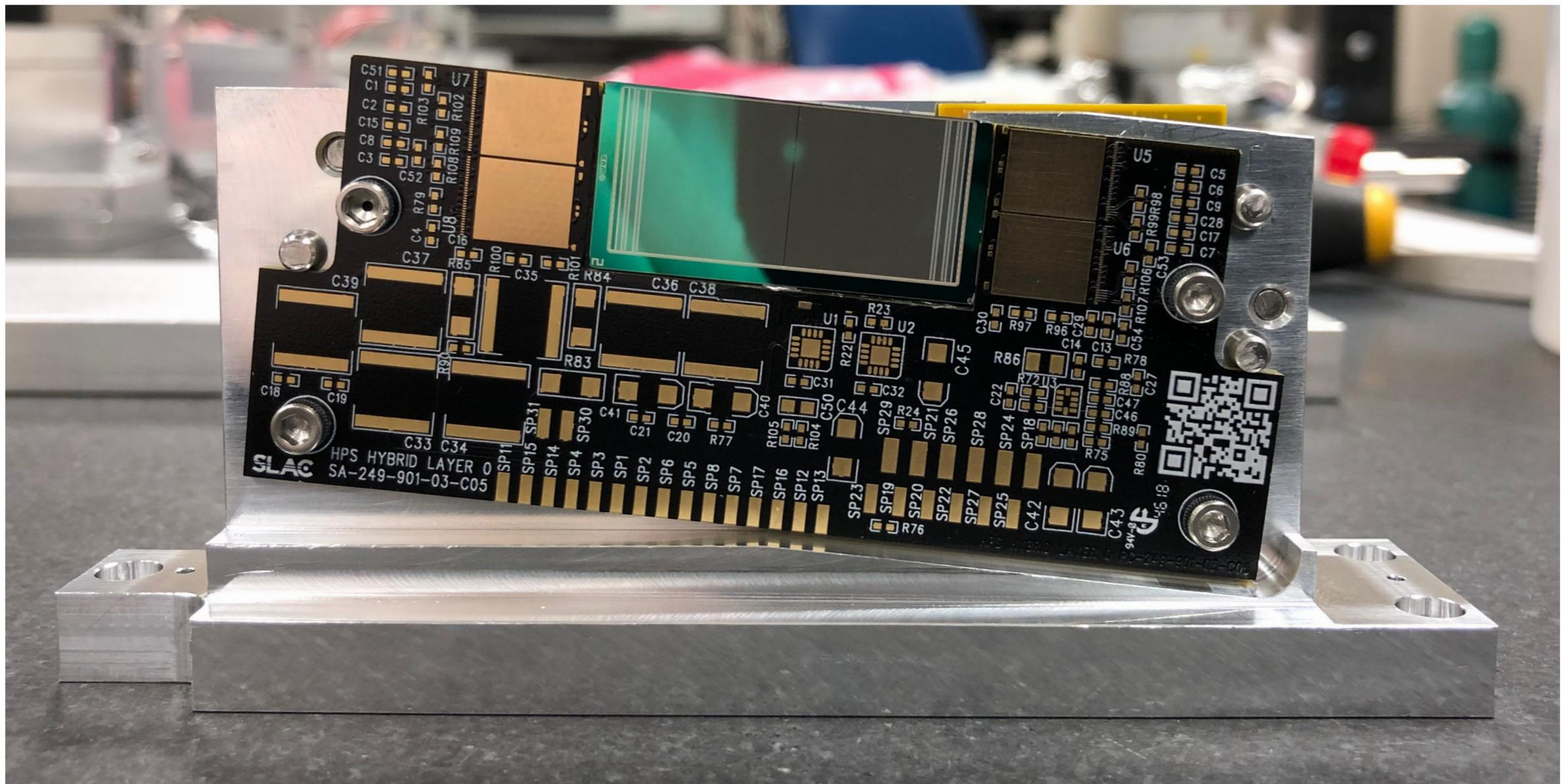
Angular acceptance of cooling block begins at 300 mrad, outside of SVT acceptance and where rate of brems is suppressed by  $>6$  orders of magnitude.
