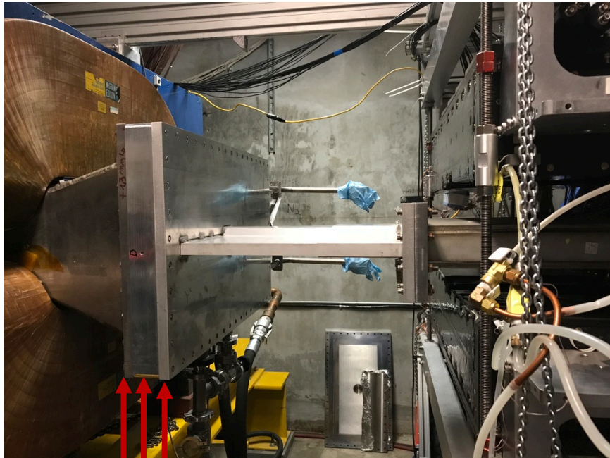
↑ Ecal vacuum chamber flange ↑ Hodoscope flange ↑ SVT vacuum chamber flange
