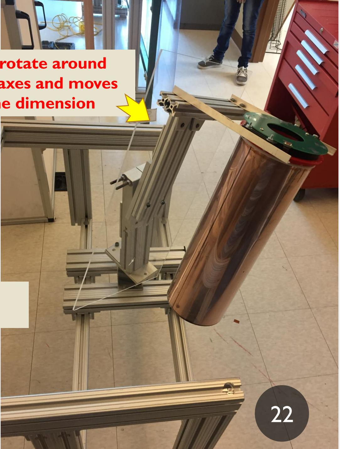
**Can rotate around two axes and moves in one dimension**
