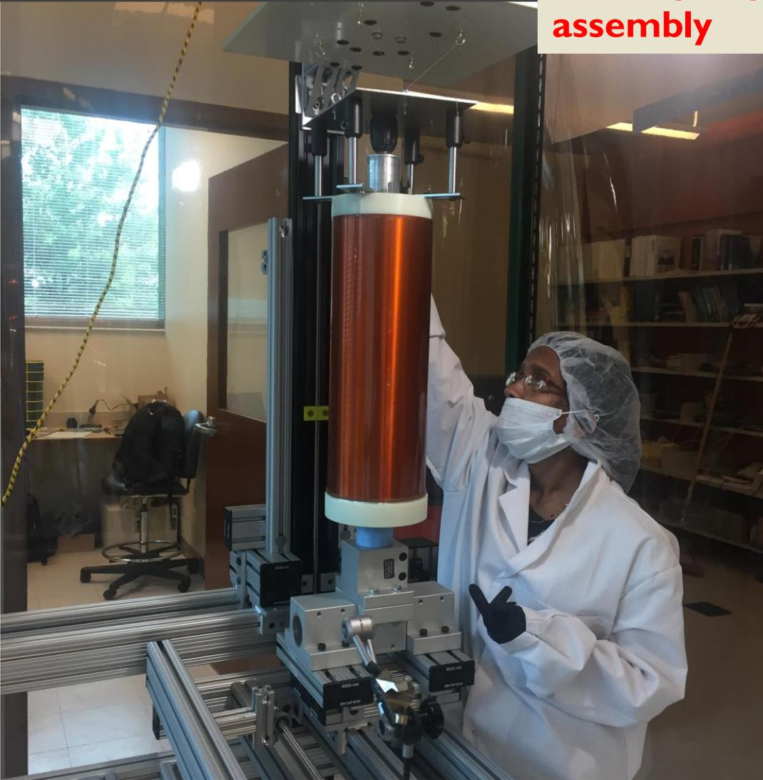
**Removal of glued capton cylinder using puller mechanism**
