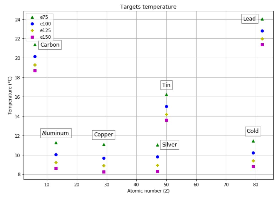
Fig 5: Targets maximum temperature plot for the 4 different conductive ribbon thickness.
