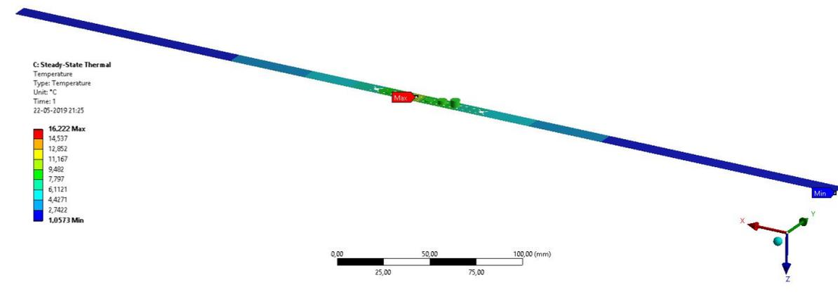
Fig 4: Ribbon with carbon, aluminum, copper, tin, lead, silver and gold targets. The beam is in the tin target.
