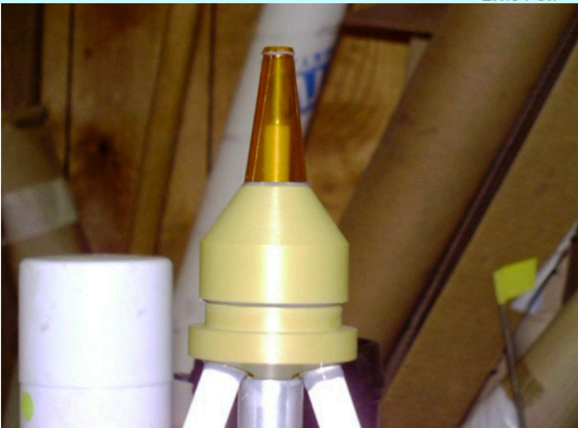
**Fig. 2.** A photograph of the cryotarget cell assembly, showing the cryotarget base, standoff, and outer cone with lap joint fabrication.
