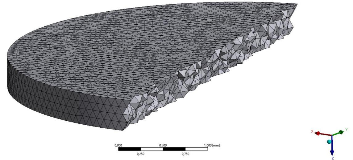
Fig 1: Copper target section plane discretization.
