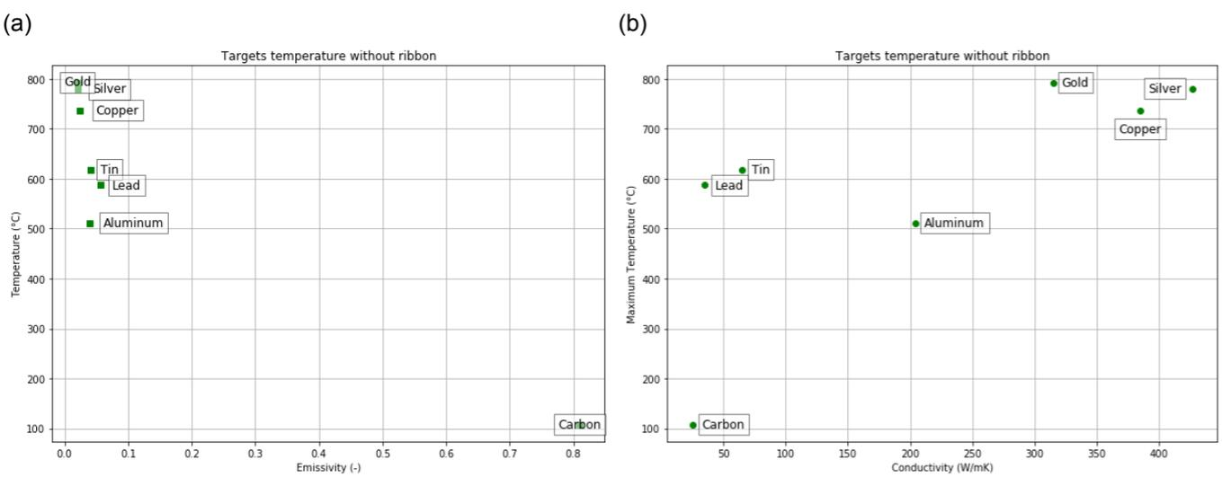
Fig 3: Targets temperature plots. (a) Target maximum temperature vs target emissivity. (b) Target maximum temperature vs target conductivity.
