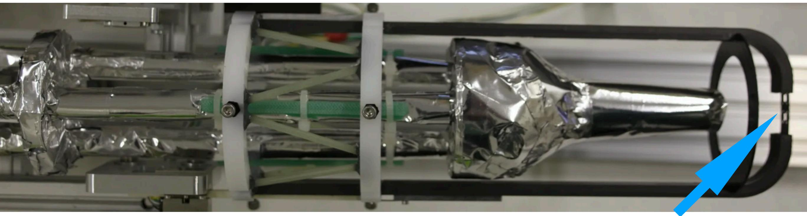
The solid targets are glued into the holes on this band. The band slides in a channel in the black outer holder, positioned by a piezoelectric motor. The radiation dose to that motor has been calculated by Lorenzo Zana, and it is well below the levels to which similar motors have been tested and found to continue operating, in published studies.
