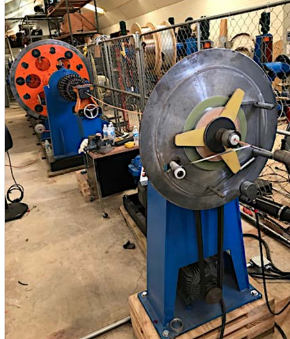
CIC manufacturing process at ATC: a) 24-spool stranding machine; b) SS foil over-wrap Drawing of sheath onto cable Completed 125 m length of CIC.
