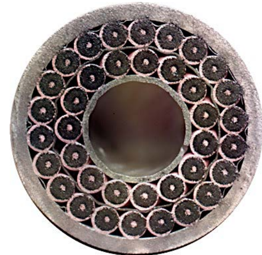
Sample of 2-layer CIC, bent on 61 mm bend radius.
