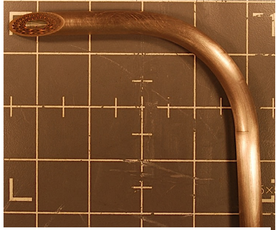
Sample of 2-layer CIC, bent on 61 mm bend radius.
