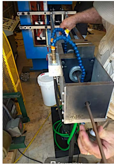
CIC manufacturing process at ATC: a) 24-spool stranding machine; b) SS foil over-wrap Drawing of sheath onto cable Completed 125 m length of CIC.
