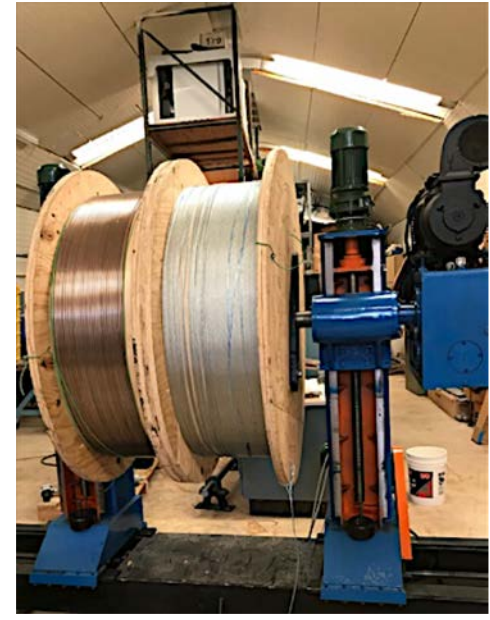
CIC manufacturing process at ATC: a) 24-spool stranding machine; b) SS foil over-wrap Drawing of sheath onto cable Completed 125 m length of CIC.
