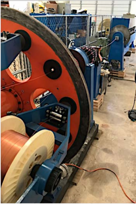
CIC manufacturing process at ATC: a) 24-spool stranding machine; b) SS foil over-wrap Drawing of sheath onto cable Completed 125 m length of CIC.
