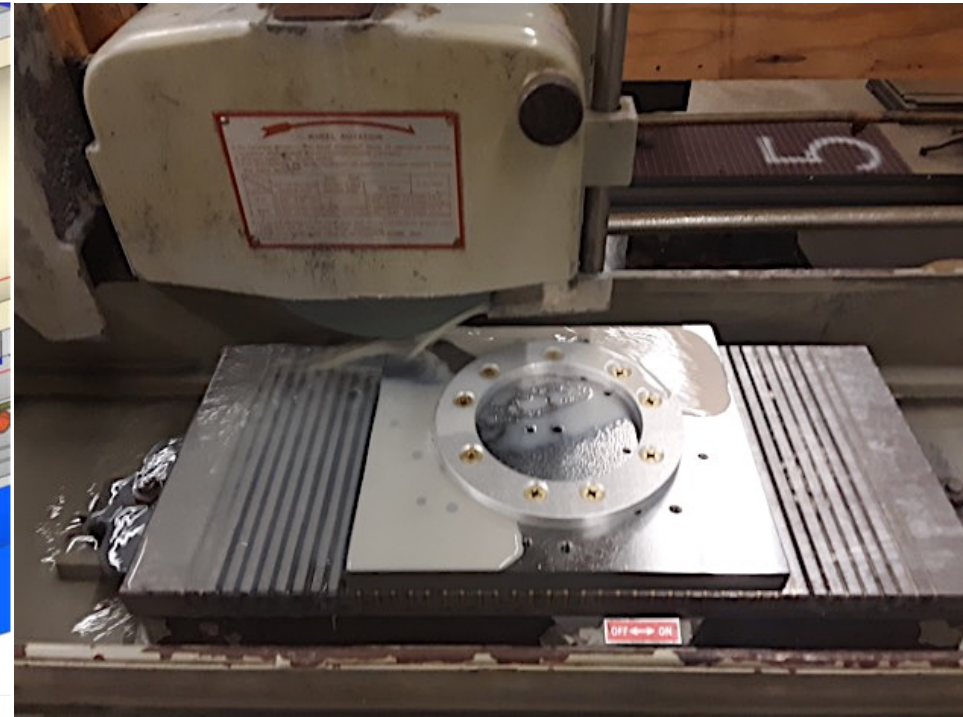
Aluminum spacer ring mounted on a steel base plate and locked to the magnetic chuck of the surface grinder.
