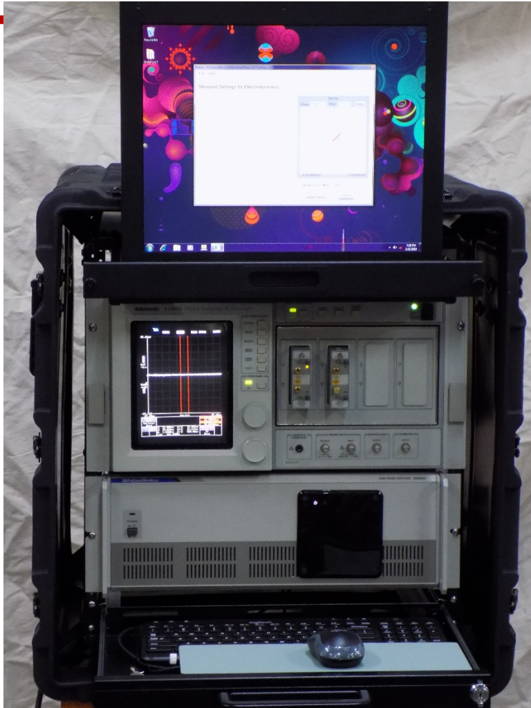
Electrodynamics developed stand-alone HAWG with a Tektronix oscilloscope and a PC based LLRF controller
