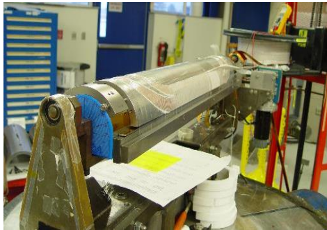
Coil winding and curing, Ceramic binder
