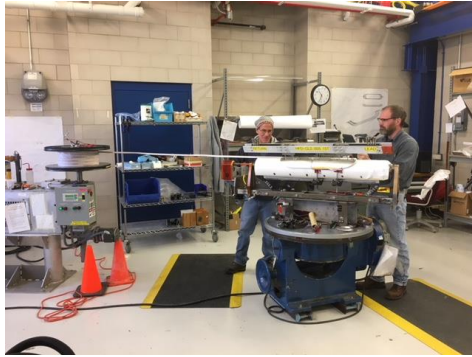
Coil winding and curing, Ceramic binder
