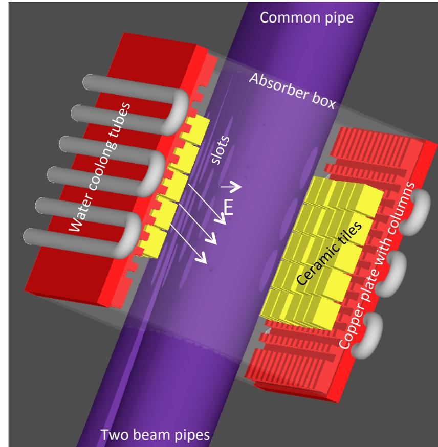
To show the how HOM absorber works we simulate two cases when ceramic tiles do not absorb HOM power (loss tangent is zero) and absorb the power.
