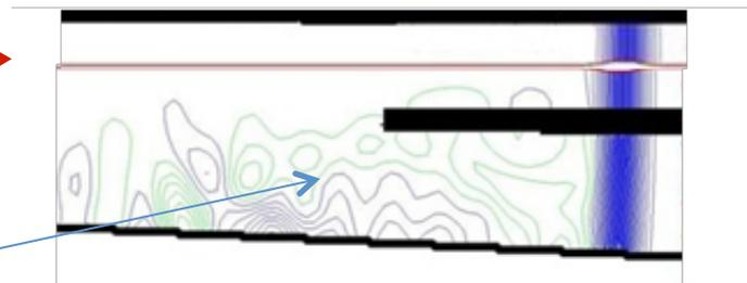
Some part of the bunch field is cut by the metal pipe connection
