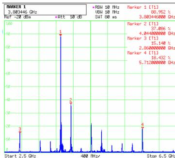
Measured single bunch and multi bunch spectrum
