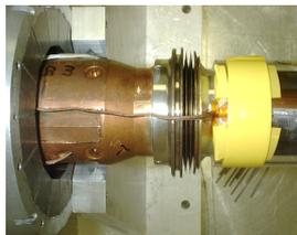
To determine if any single HOM resonance was responsible for the heating, the RF phase of the HER was then moved relative to the LER and a modulation of the temperature was measured. The resonance was around 5.4 GHz. S. Ecklund et al., "High Order Mode Heating Observations", PAC'2001, p.3576.
