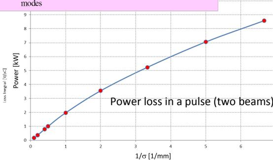
Power loss due to resistive wall.
