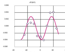
We also measured the spectrum of the fields generated in the interaction region and found one mode at the frequency of 5.59 GHz, the amplitude of which was correlated with the heating power, calculated from the bellows temperature and cooling time. A. Novokhatski "HOM effects in vacuum chamber with short bunches", PAC 2005.
