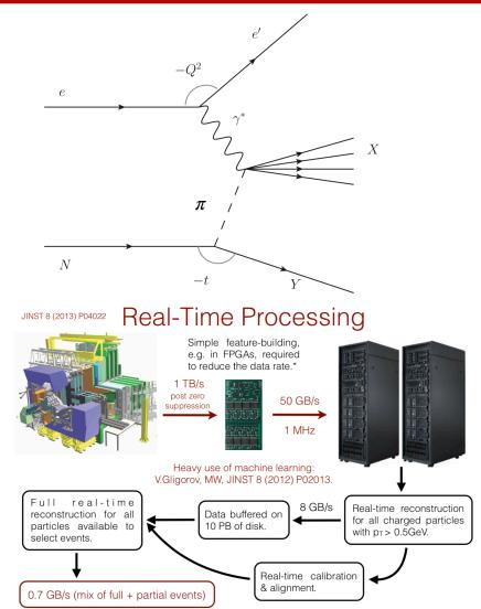
\*LHCb will move to a triggerless-readout system for LHC Run 3 (2021-2023), and process 5 TB/s in real time on the CPU farm.
