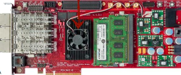
PCIe Gen2, 8 Lanes 8x 5.0 Gbps, connected to Xilinx PCIe Hard Block
