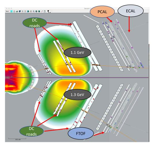
The trigger is 99% efficient for CLAS12 kinematics
