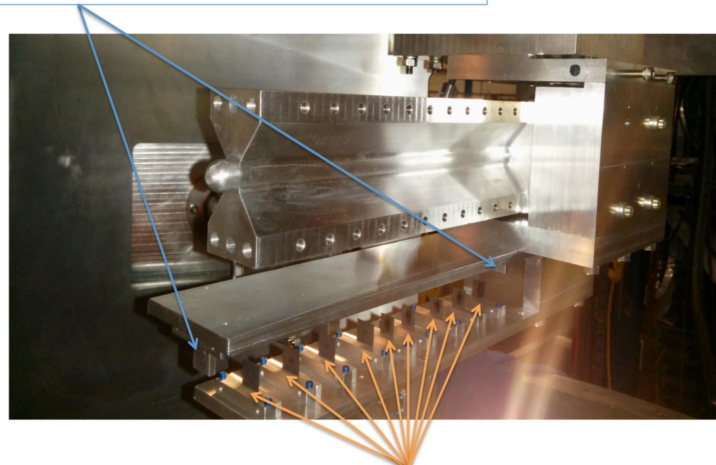
Optical target: a series of foils of carbon (9) to check the alignment of target and spectrometers (optics)
