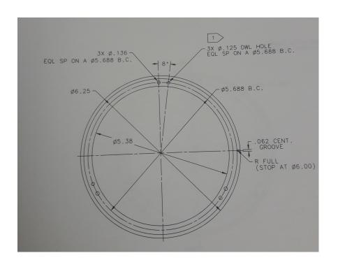
Mount will be modified to include EPR RF coil underneath NMR RF coil (~ 5.38")
