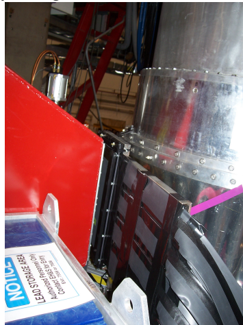
Forward tracker in position between Cherenkov snout and target OVC
