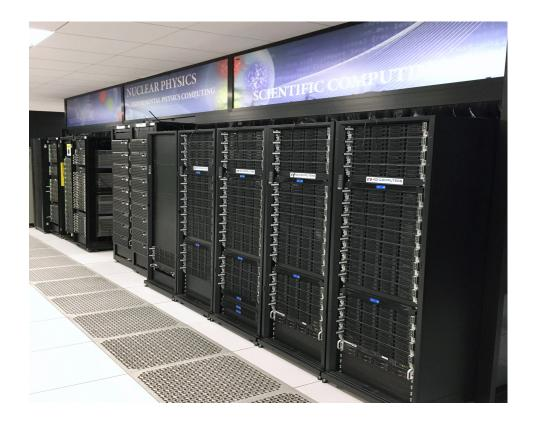
Xeon Phi 7230, 64 cores/node, 264 nodes
