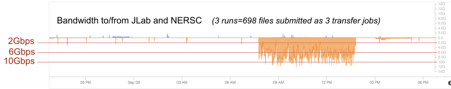
Figure 5: Screen capture of bandwidth usage between JLab and NERSC during a bandwidth test. During this test, 698 files, each 20GB in size was transferred from JLab to NERSC using 3 transactions of 4.6TB each (total of 14TB).
