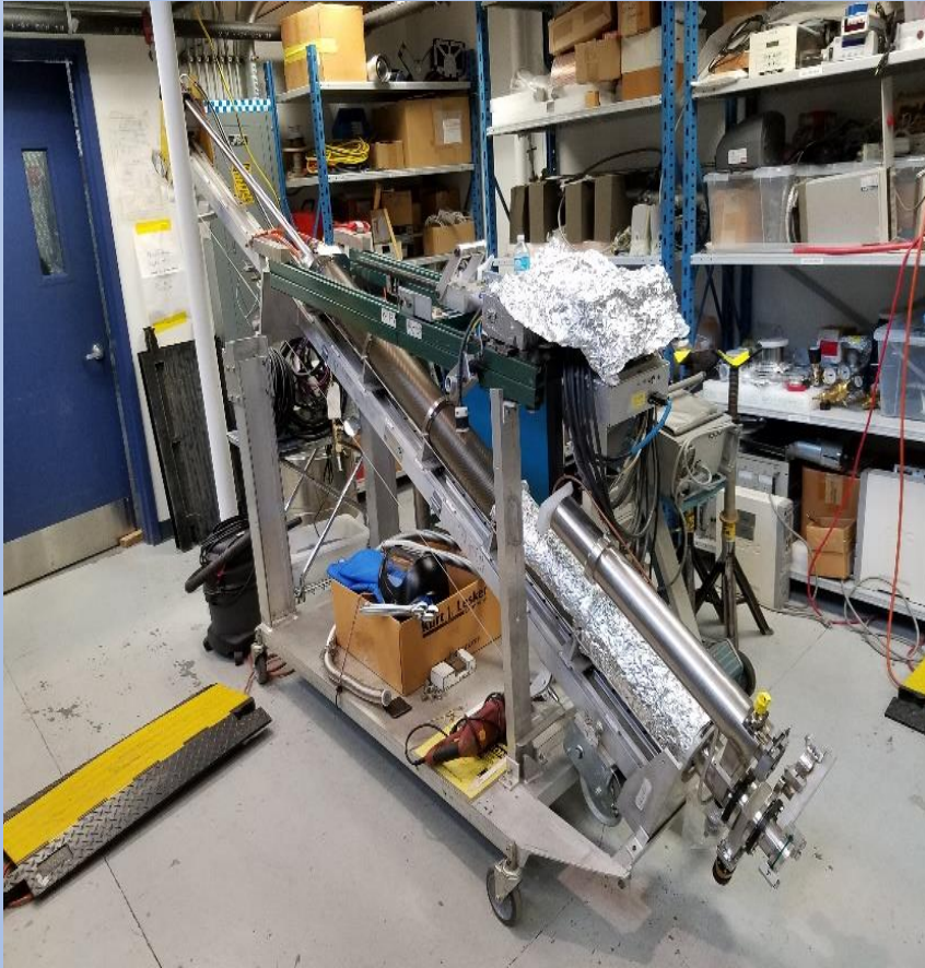
Transfer Cryostat (TC) – a cryostat used to transfer targets between cryostats with a temperature of 2K and a magnetic field of 0.1 T.
