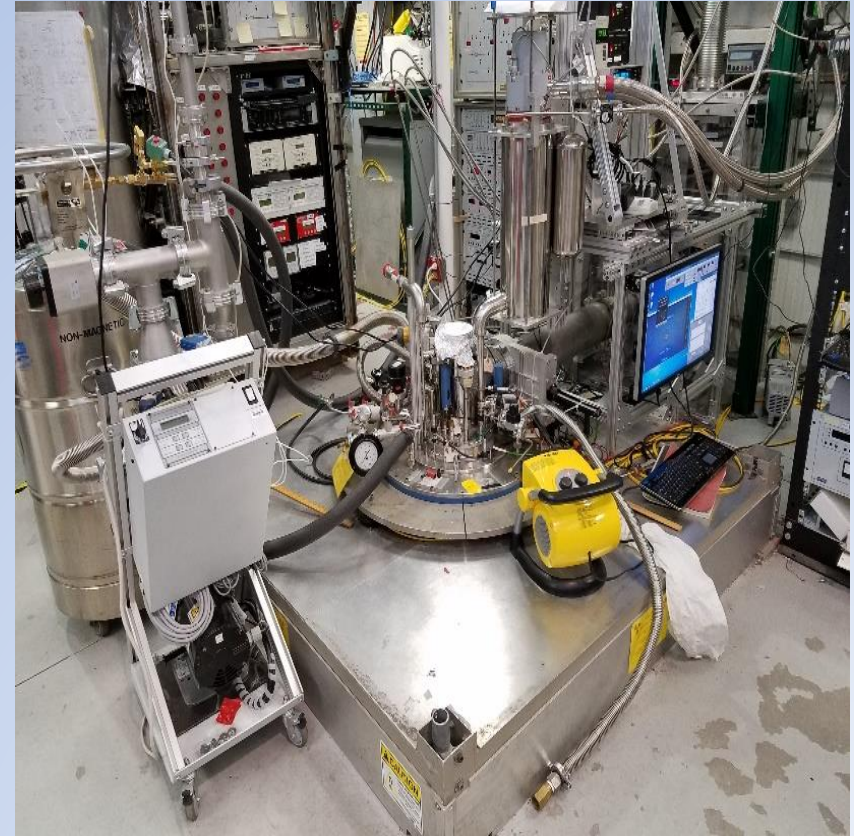
Dilution Refrigerator (DF) – a cryostat used to polarize targets with a temperature of 10 mK and a magnetic field of 15 T.
