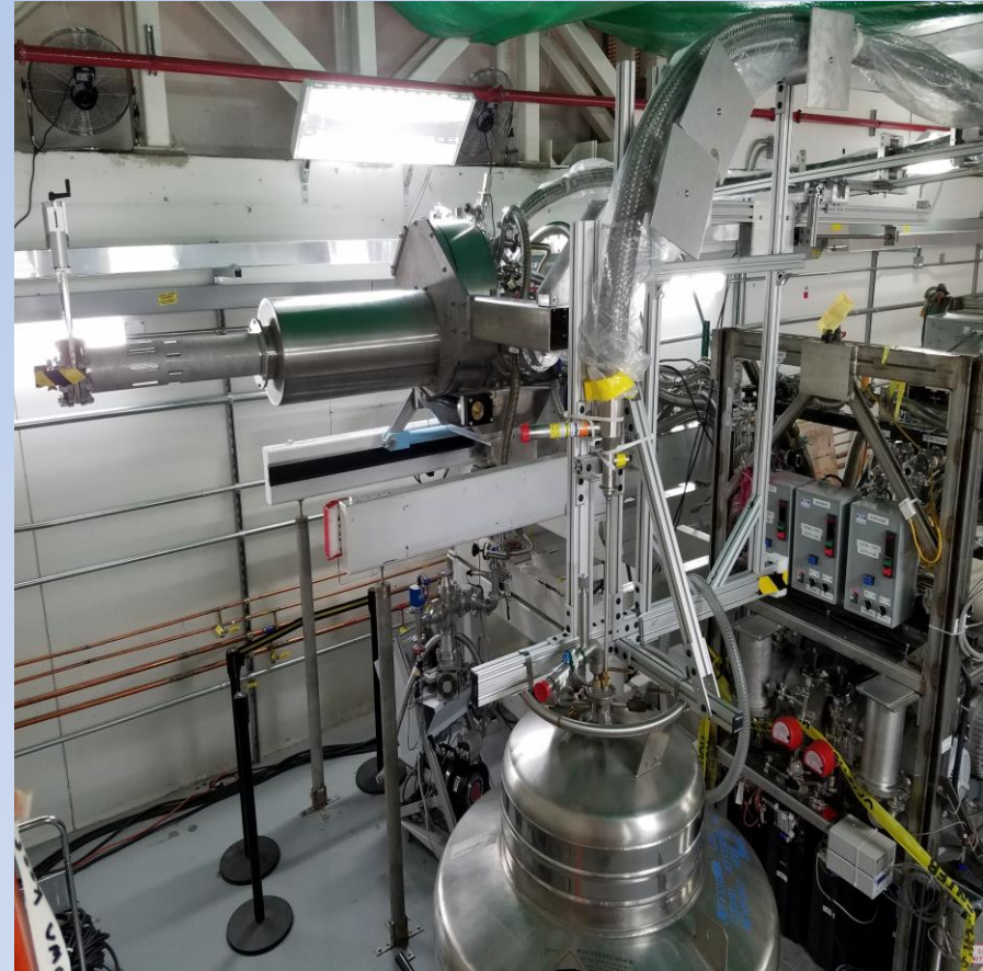
In-Beam Cryostat (IBC) – a cryostat used to operate the target under a particle beam with a temperature range of 50 mK to 300 mK, a longitudinal magnetic field up to 0.9 T, and a transverse magnetic field up to 0.07 T
