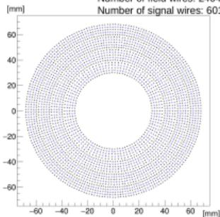
With usual gold plated tungstate wires, to ensure a 20 microns sag, the total weight on the end plate due to the tension is about 600 kg.
