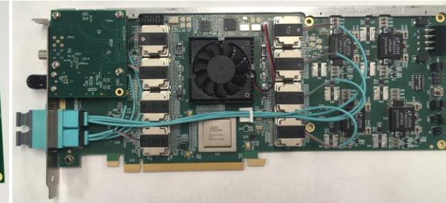
sPHENIX SAMPA+FELIX DAQ chain reading out EIC GEM detectors
