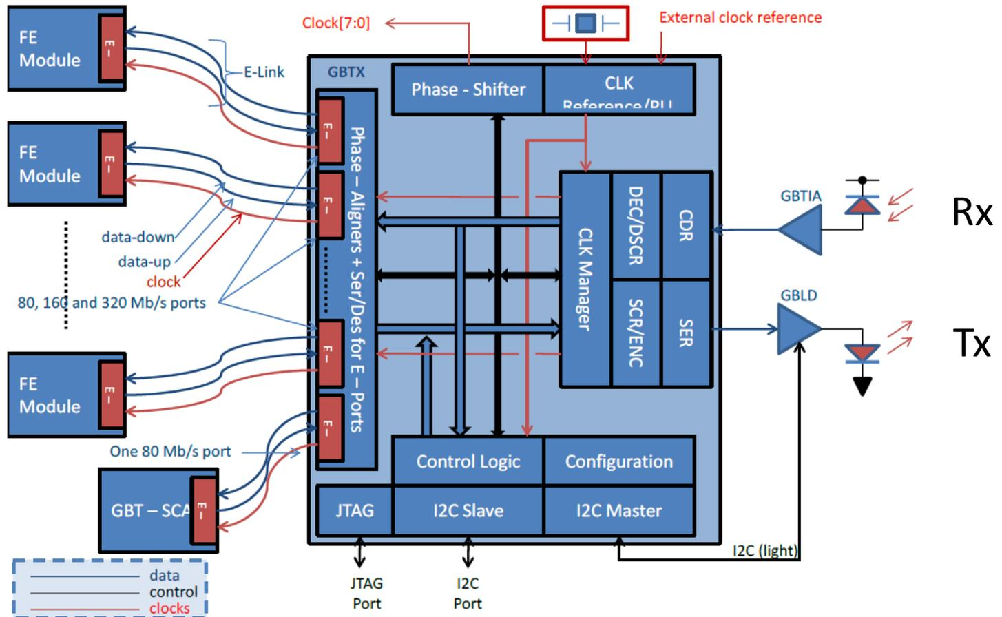
E-Link - Electrical serial link (SLVS)
