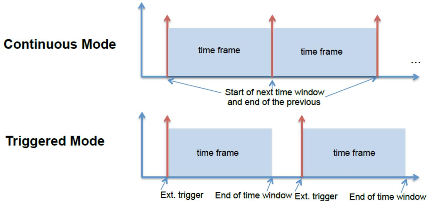
Time frame is programmable (max = 1024 ADC samples)
