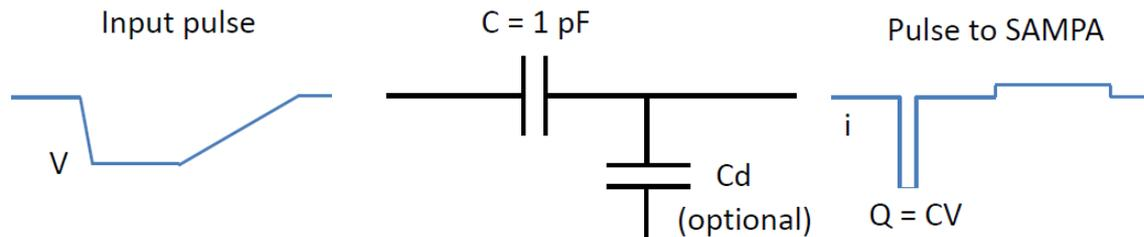
SAMPA linear range  $Q < 100 \text{ fC}$  ( $V < 100 \text{ mV}$ )
