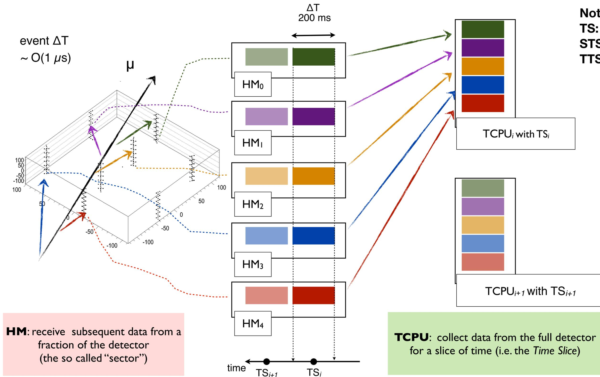
**HM:** receive subsequent data from a fraction of the detector (the so called "sector")
