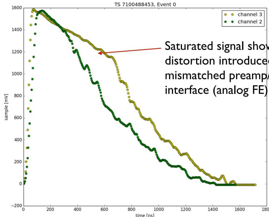
Saturated signal shows the distortion introduced by the mismatched preamp/FEM interface (analog FE)
