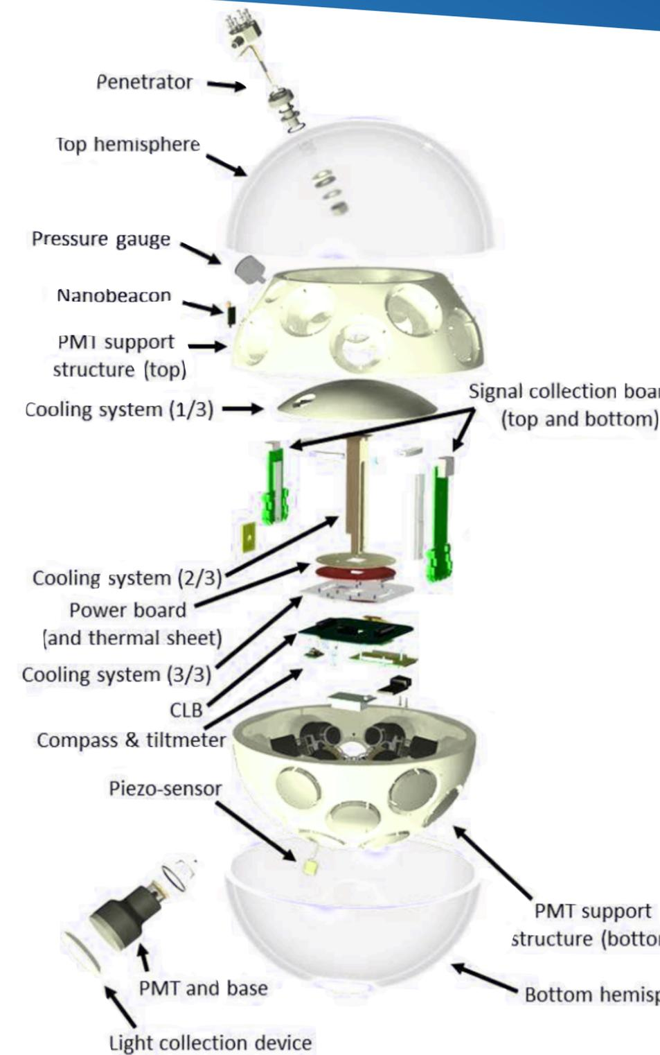
Each **DOM** implements a dedicated FPGA firmware for DAQ with an embedded software for slow-control. Communication is set via **1Gbps ethernet** connection to shore. DOMs are the **submarine nodes** of the full DAQ LAN (>10 GbE on-shore).
