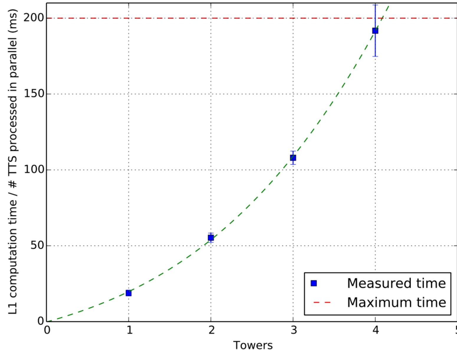
It means that for  $N > 4$  Towers additional TCPU nodes are needed (or more trigger threads, if allowed by the computing resources ).
