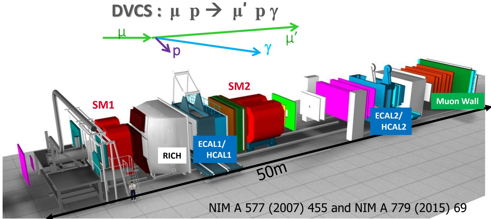
Two stage magnetic spectrometer for **large angular & momentum acceptance**
