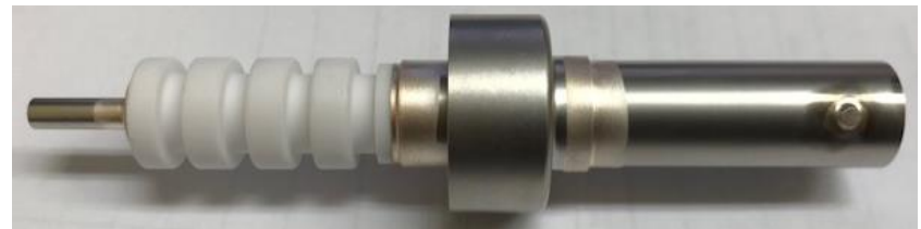
Feedthroughs from the APS-U Injection Kickers
