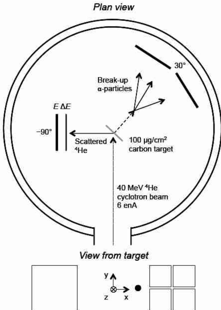
Measurement of the  $^{12}\text{C}(^4\text{He},\alpha)3\alpha$  reaction at 40 MeV in complete kinematics;
