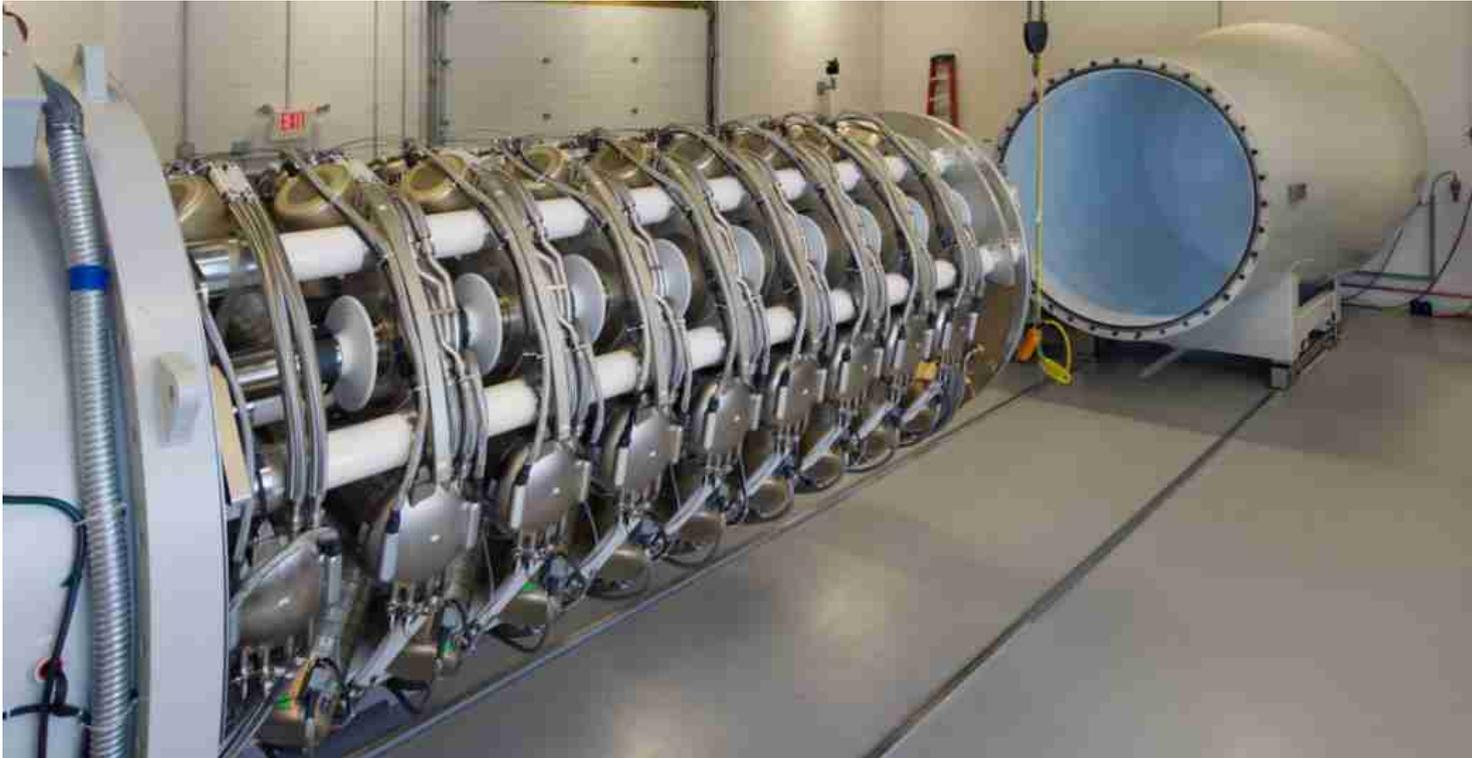
Hyperion: A single-ended electrostatic accelerator, 50 mA+ capability
