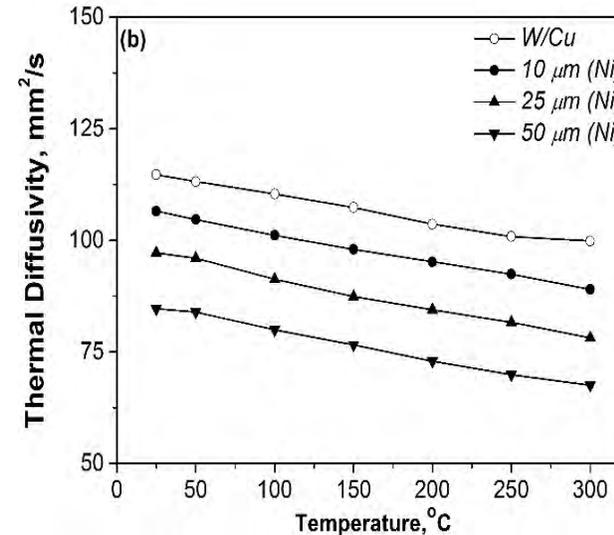
Thermal diffusivity of joined W/Al/Cu (a), W/Ni/Cu and W/Cu (b) samples
