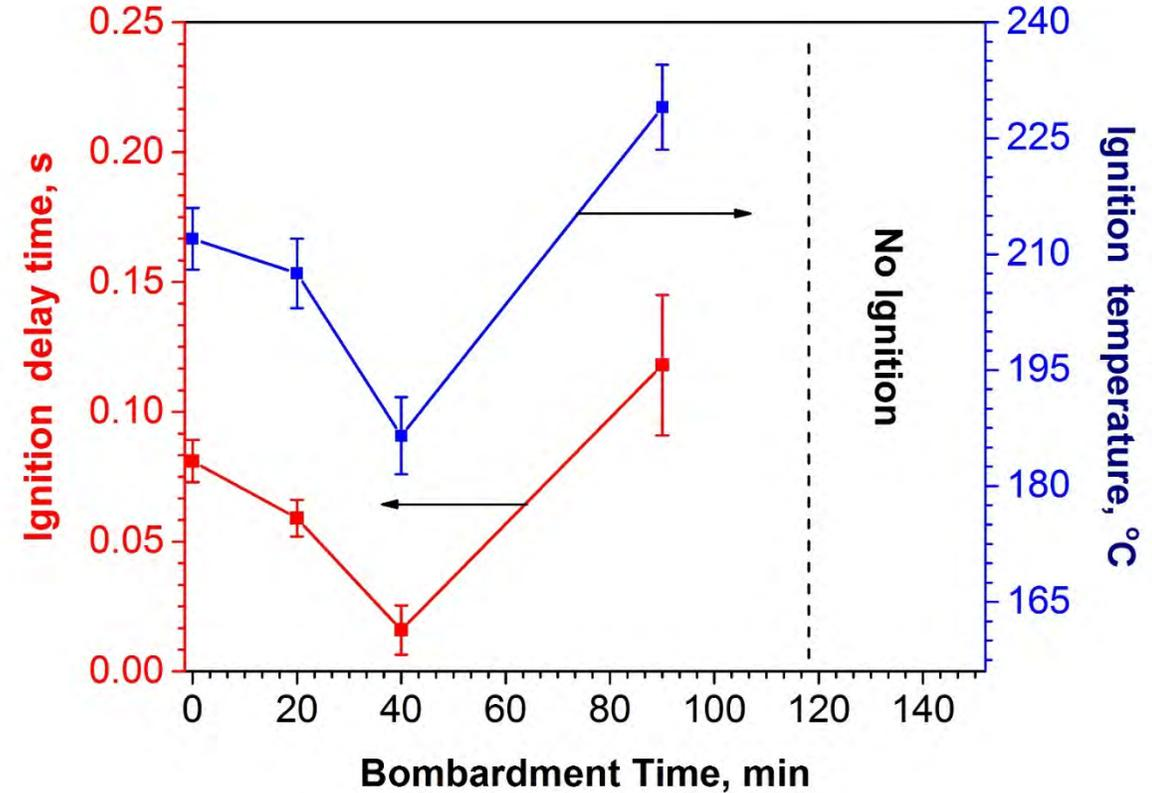
**Short-term bombardment:  $\text{Al}_3\text{Ni}$  nuclei formed in intermixed layer significantly decrease ignition temperature and ignition delay time.**
