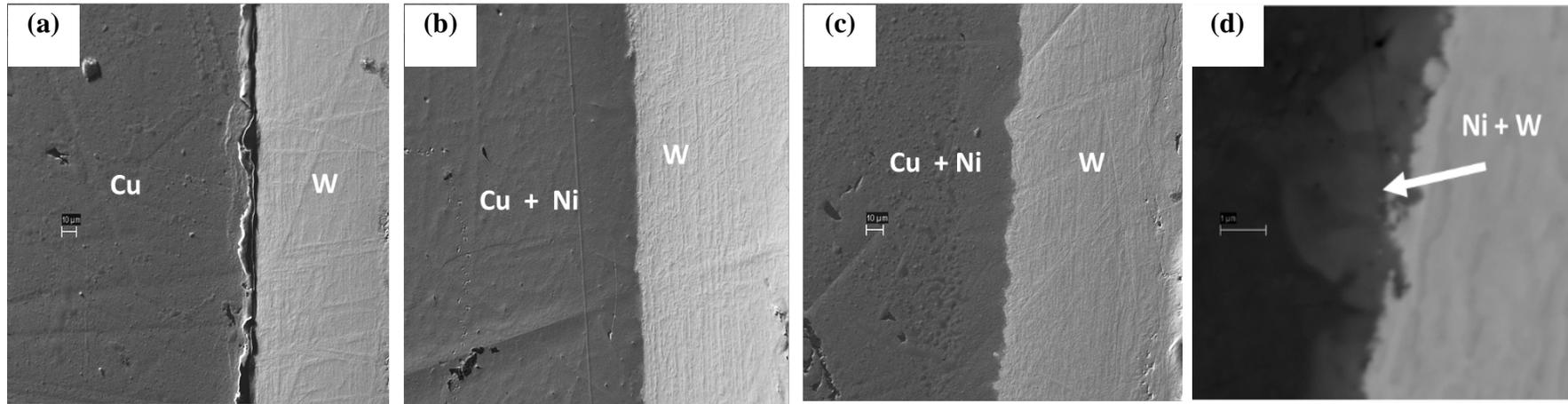
Microstructure of joined W-Cu sample: (a) without nickel of soldering layer, (b) and (c) with Ni soldering layer with 25 mm of thickness, high magnification image of Ni-W joining layer (d)
