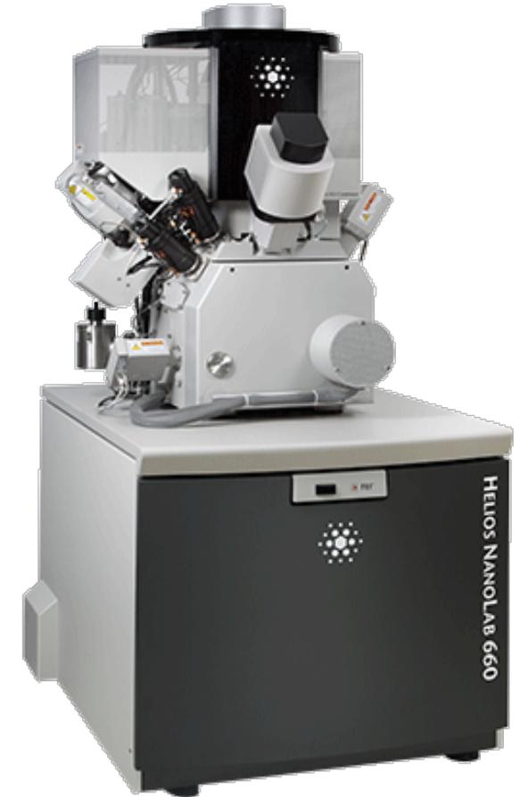
Focused Ion Beam Milling / Scanning Electron Microscopy FIB/SEM
