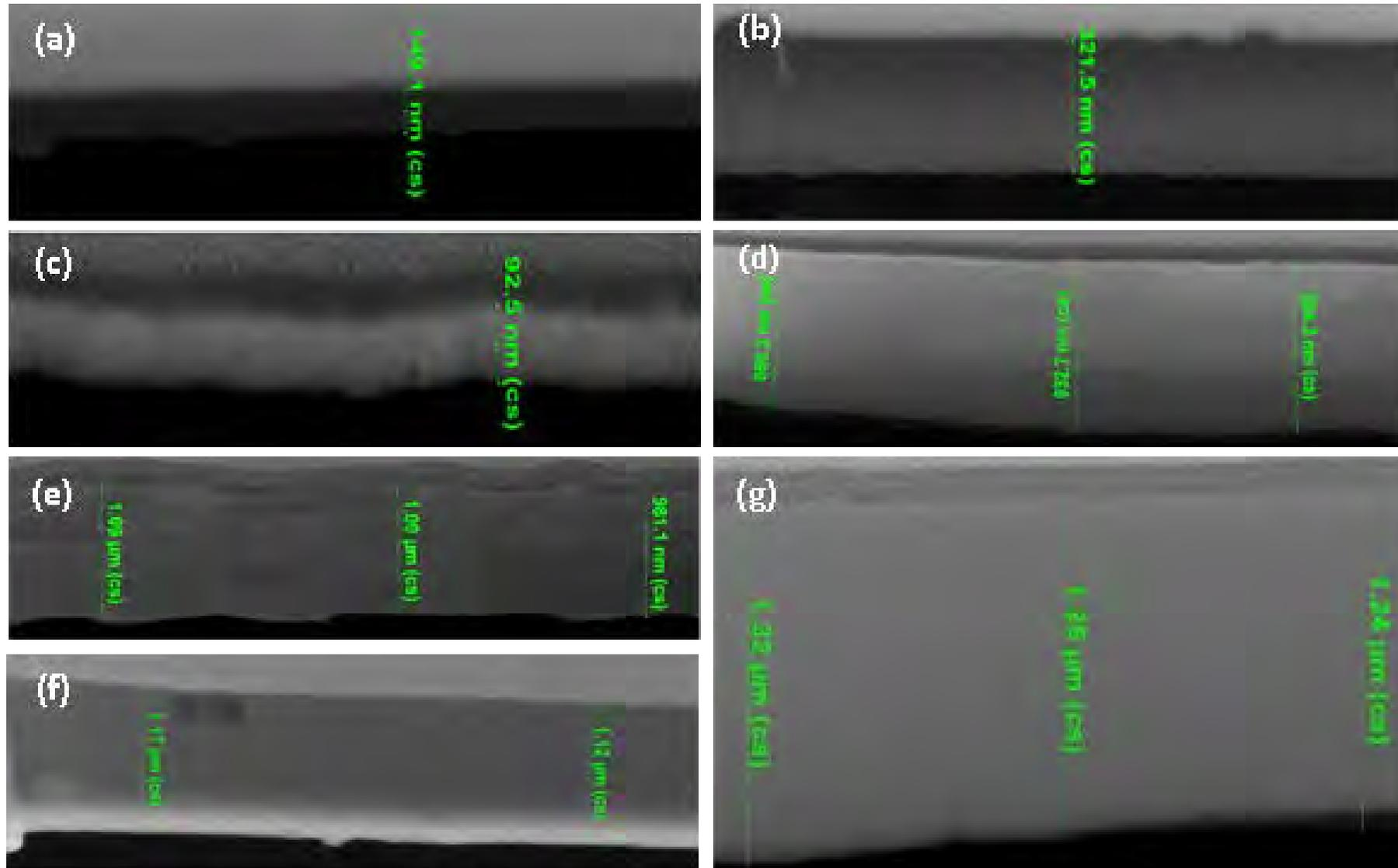
Figure 2: Cross-sectional SEM images for carbon-20(a), carbon-60 (b), gold(c), platinum (d), nickel (e), aluminum (f) and tin (g) targets
