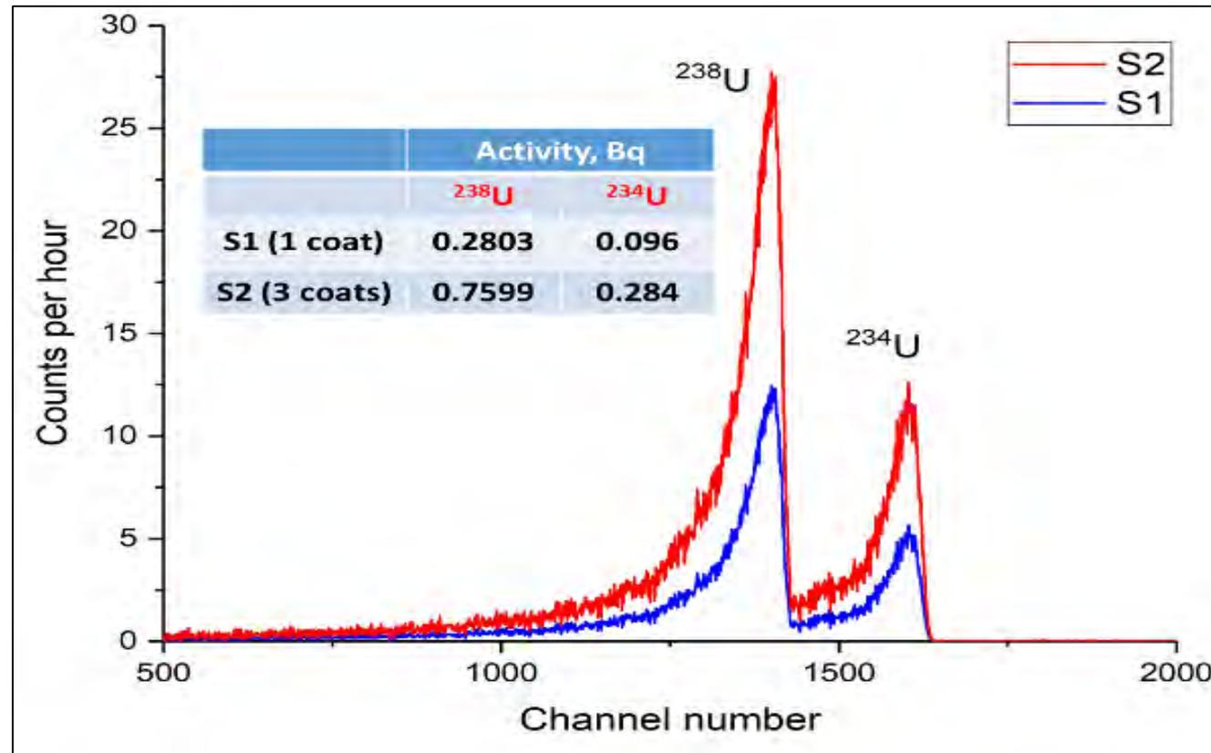
*Alpha particle counting by a silicon detector*
