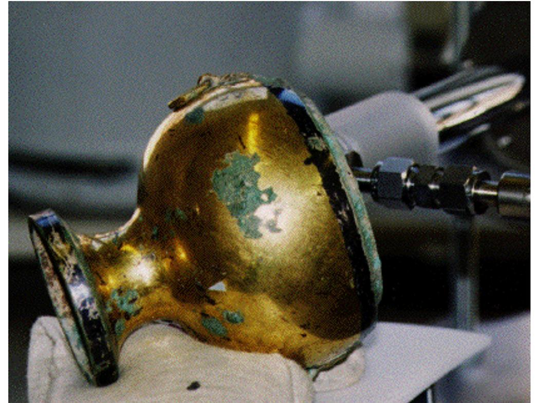
Protons transmit energy to the inner-shell electrons, ionize atoms with subsequent X-ray de-excitation
