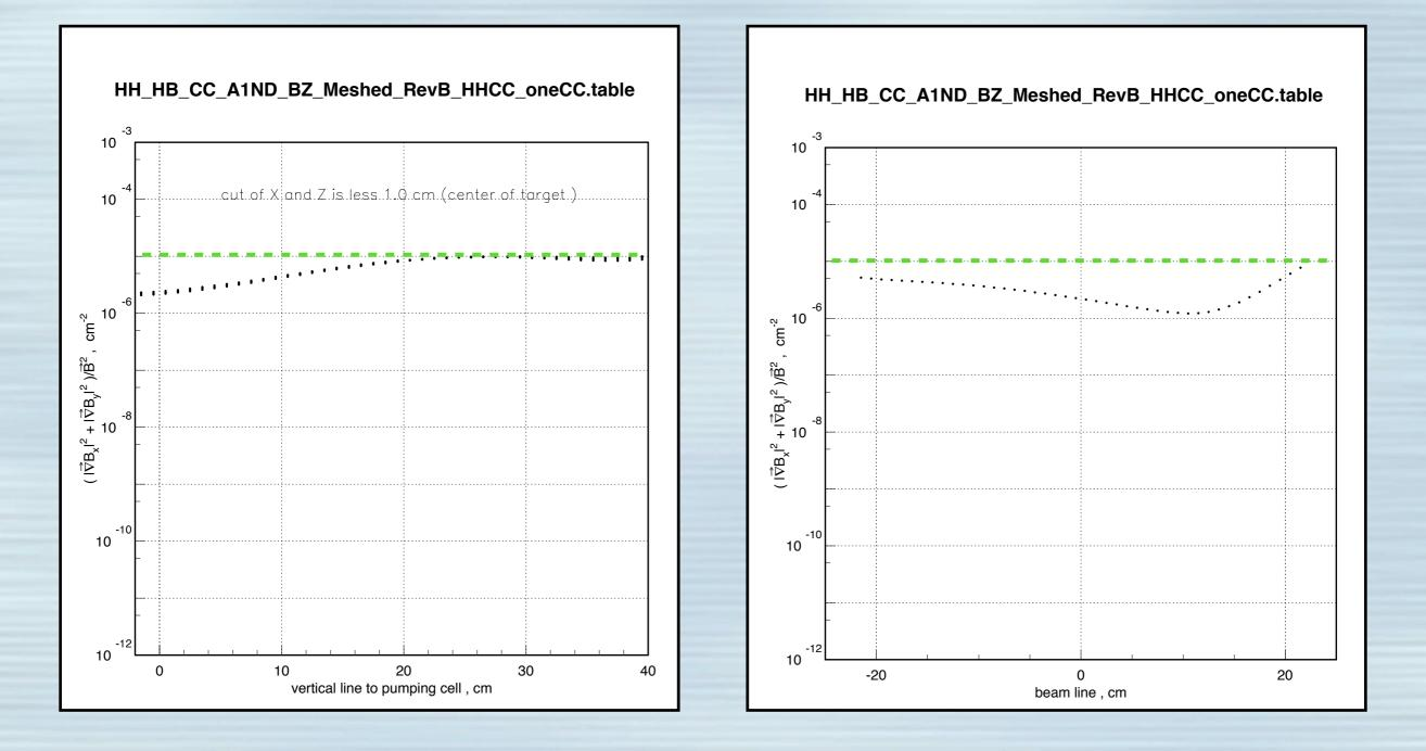
Green dotted lines indicate gradients that result in  $1/T_1 = 1/139$  hours
