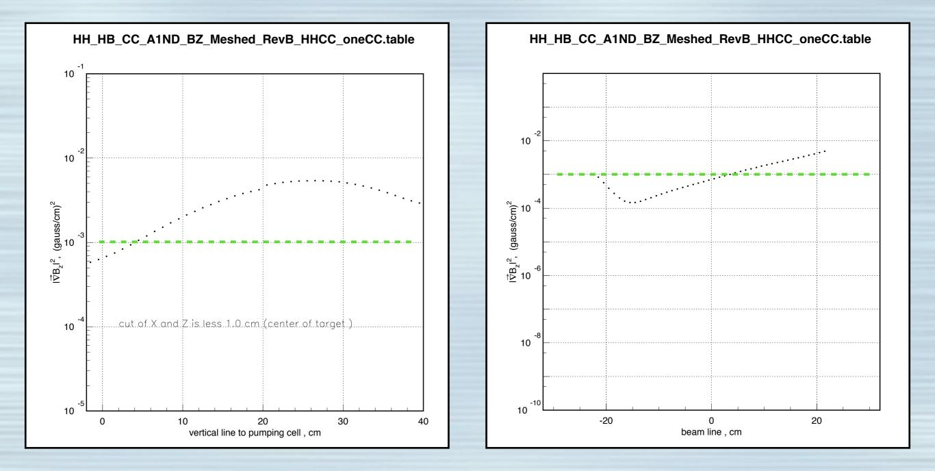
The dashed green line shows the gradient at which losses (per flip) are 0.5%.
