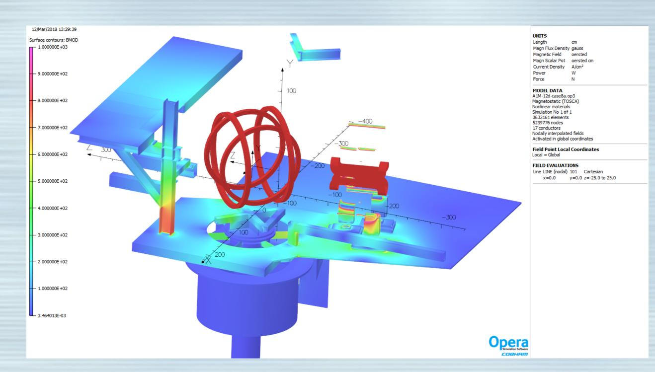
Configuration shown above is with Helmholtz coils set for longitudinal running, and the HB correction coils are not turned on (although they are for the plots I will show).
