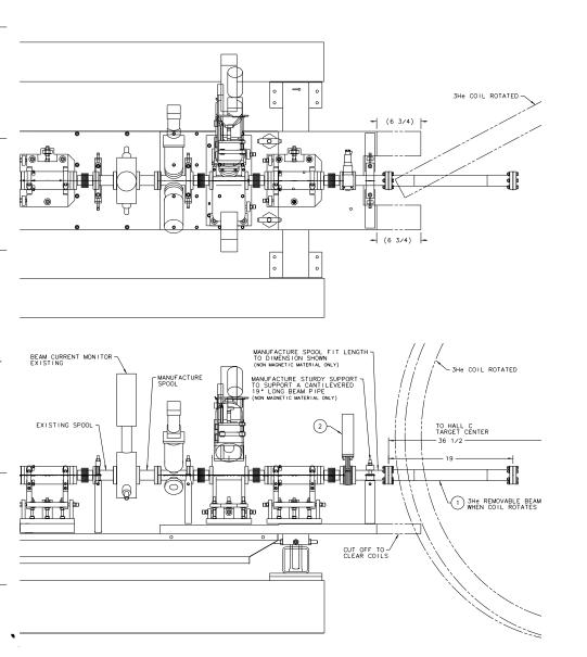
Coils for polarized <sup>3</sup>He will run into end of last girder when rotated to certain configurations
