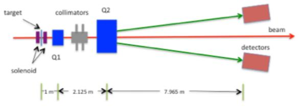
Additional large quad required to steer electrons to detectors
