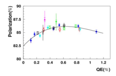
Measured QE dependence from GEp, GEp-2gamma
