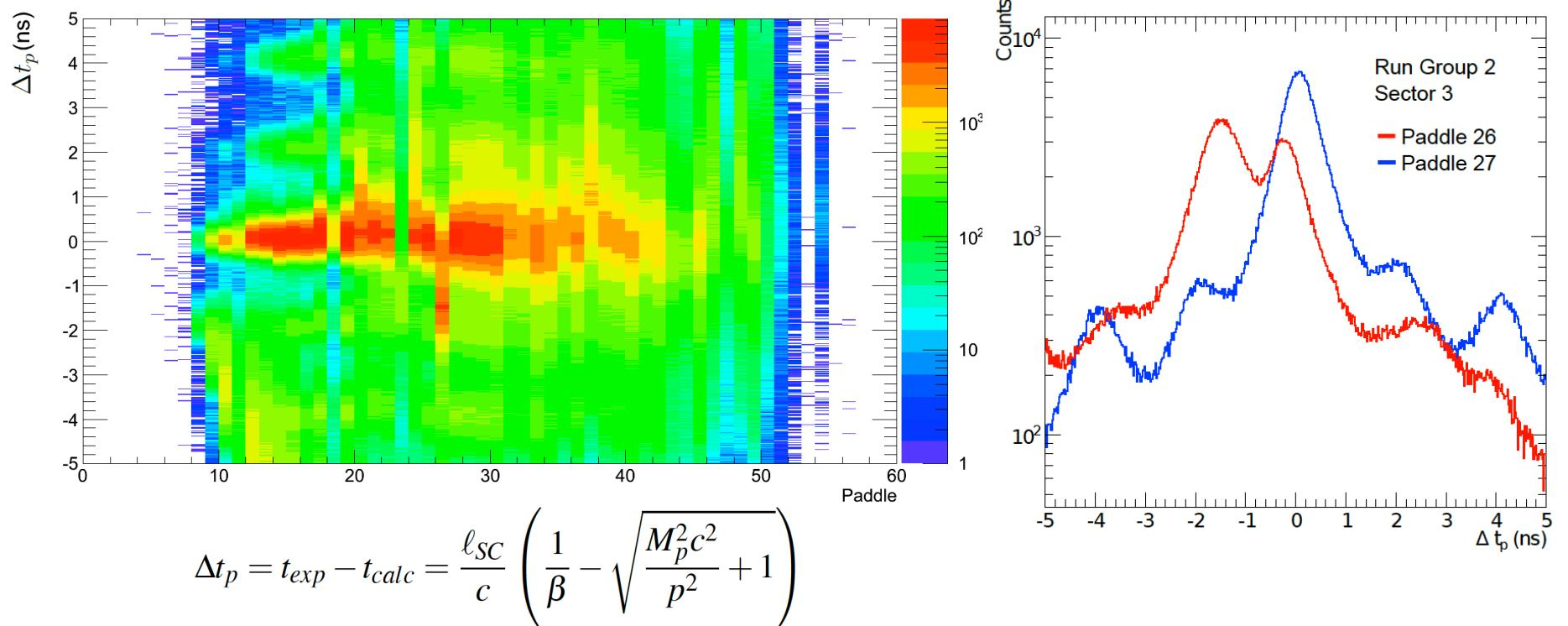
The performance of all TOF paddles has been examined by checking  $\Delta t_p$  of each paddle for each run group to reduce the probability of particle misidentification. Problematic paddles were removed from the analysis.
