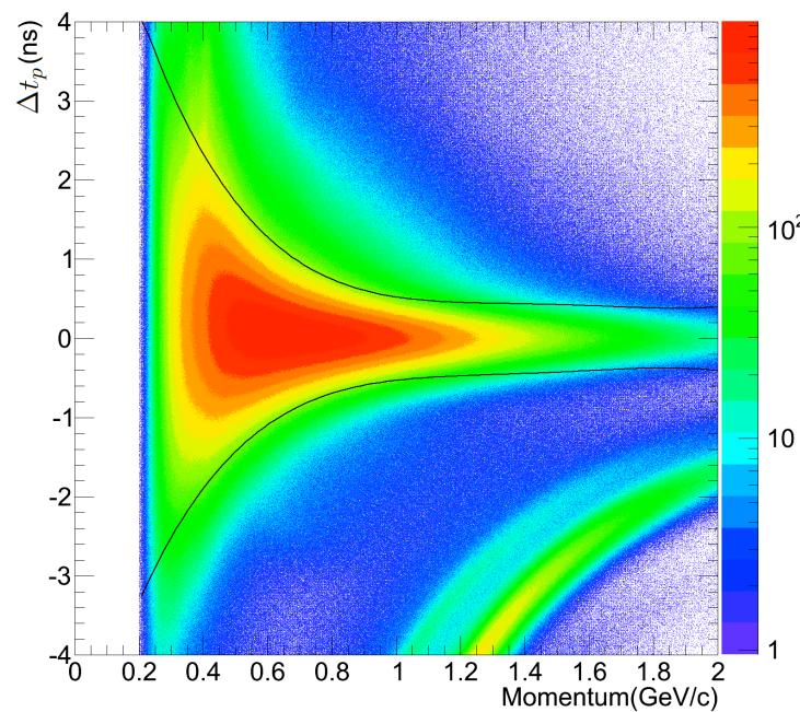
The photon that initiated the reaction and was coincident with the detected proton was selected by using the CLAS-tagger coincidence time.
