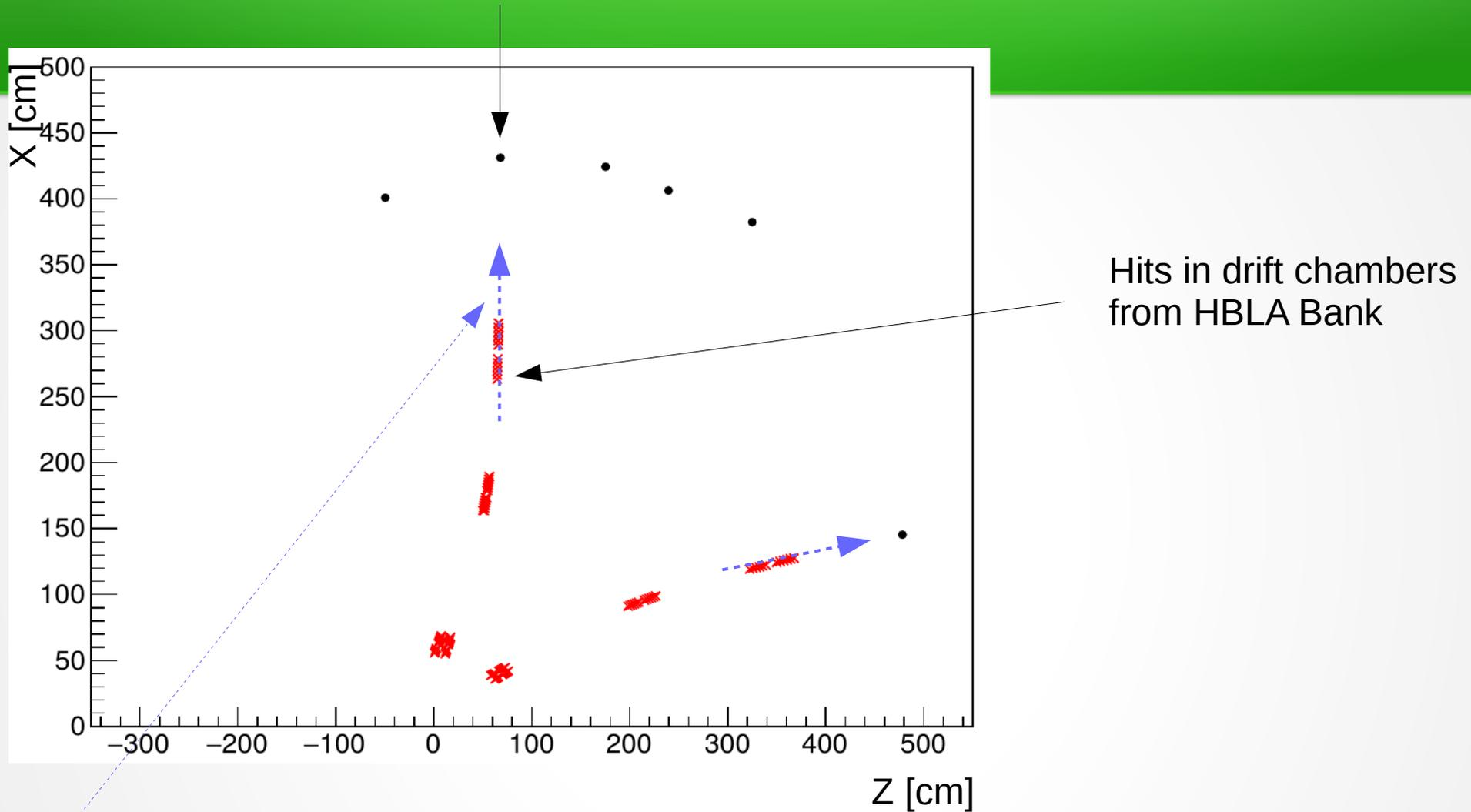
Fit the track direction based on the hits in super layer (34 layers)
