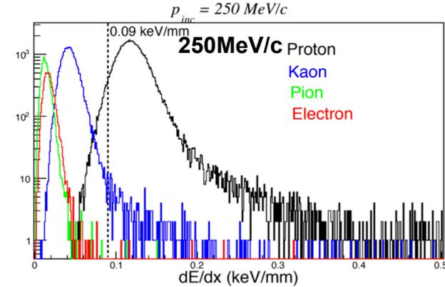
Energy deposit in He of original RTPC for different particles
