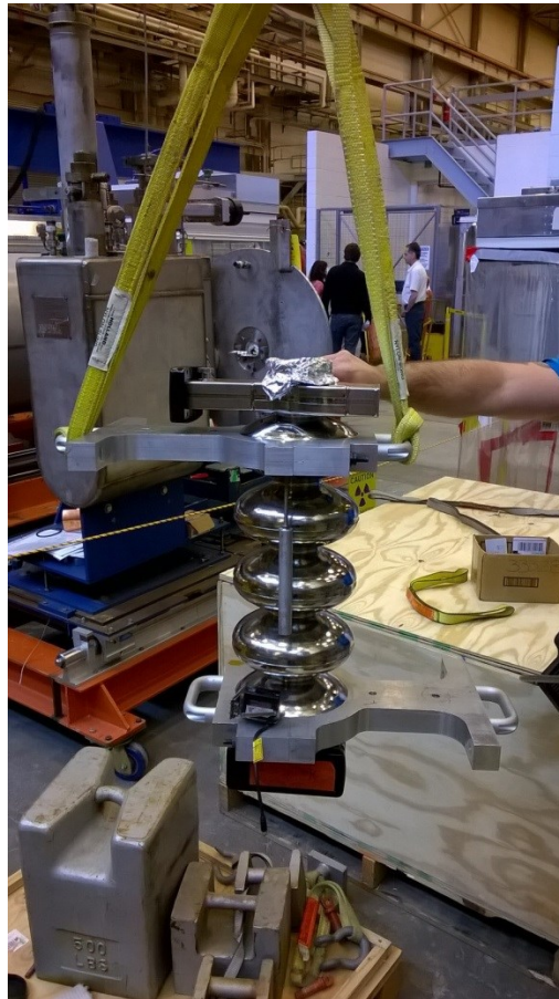
Fig. 8. Setup for measuring the stiffness of both C20/C50 and C75 cavities.
