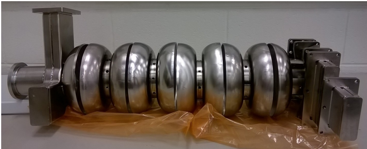
Figure 8. Dumb-bells and end-groups with end half-cells for 5C75-003 prior to machining the weld-preps on the dumb-bells' equators, cleaning and EB welding..
