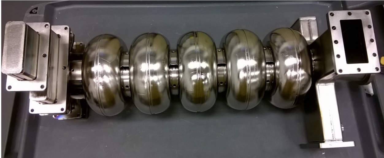
Figure 10. Picture of the fully welded 5C75-003 cavity.
