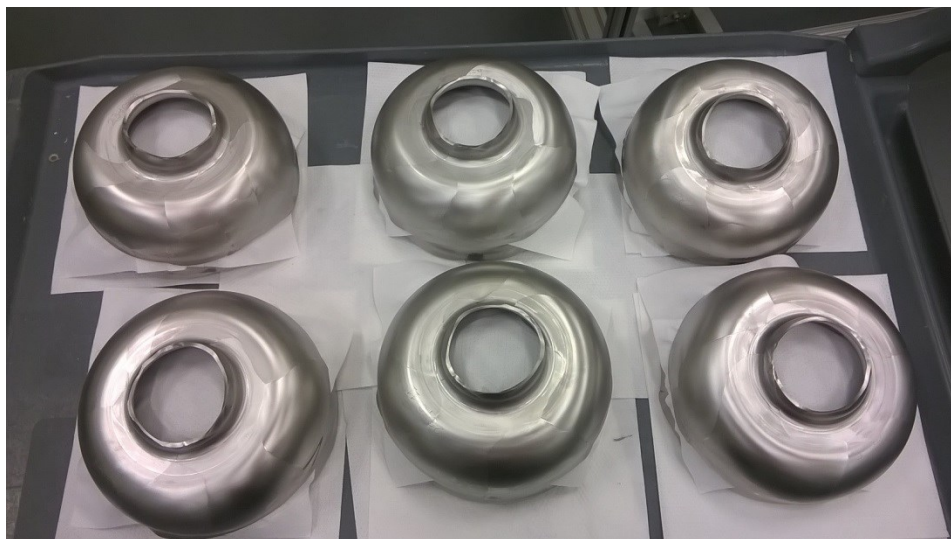
Figure 4. Set of half-cells used to fabricate 5C75-001 after stamping.
