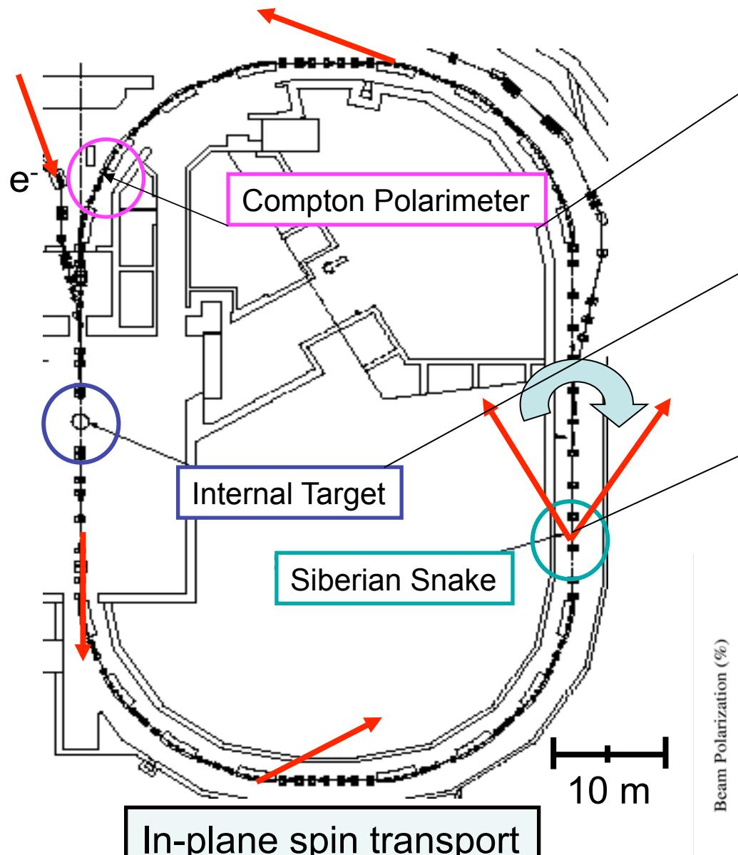
Monitoring of electron beam polarization
