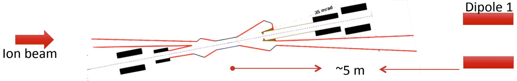
Electron-beam axis: Solenoid axis must align with electron beam
