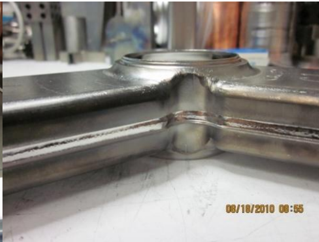
CNC machine two halves and EBW
