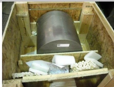
RRR>250 large grain Nb ingot
