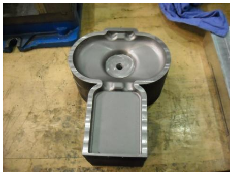
Finished first half with 4mm wall thickness
