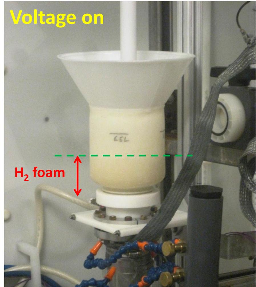
Thick hydrogen foam layer was built up on top of electrolyte during VEP voltage on so far.
