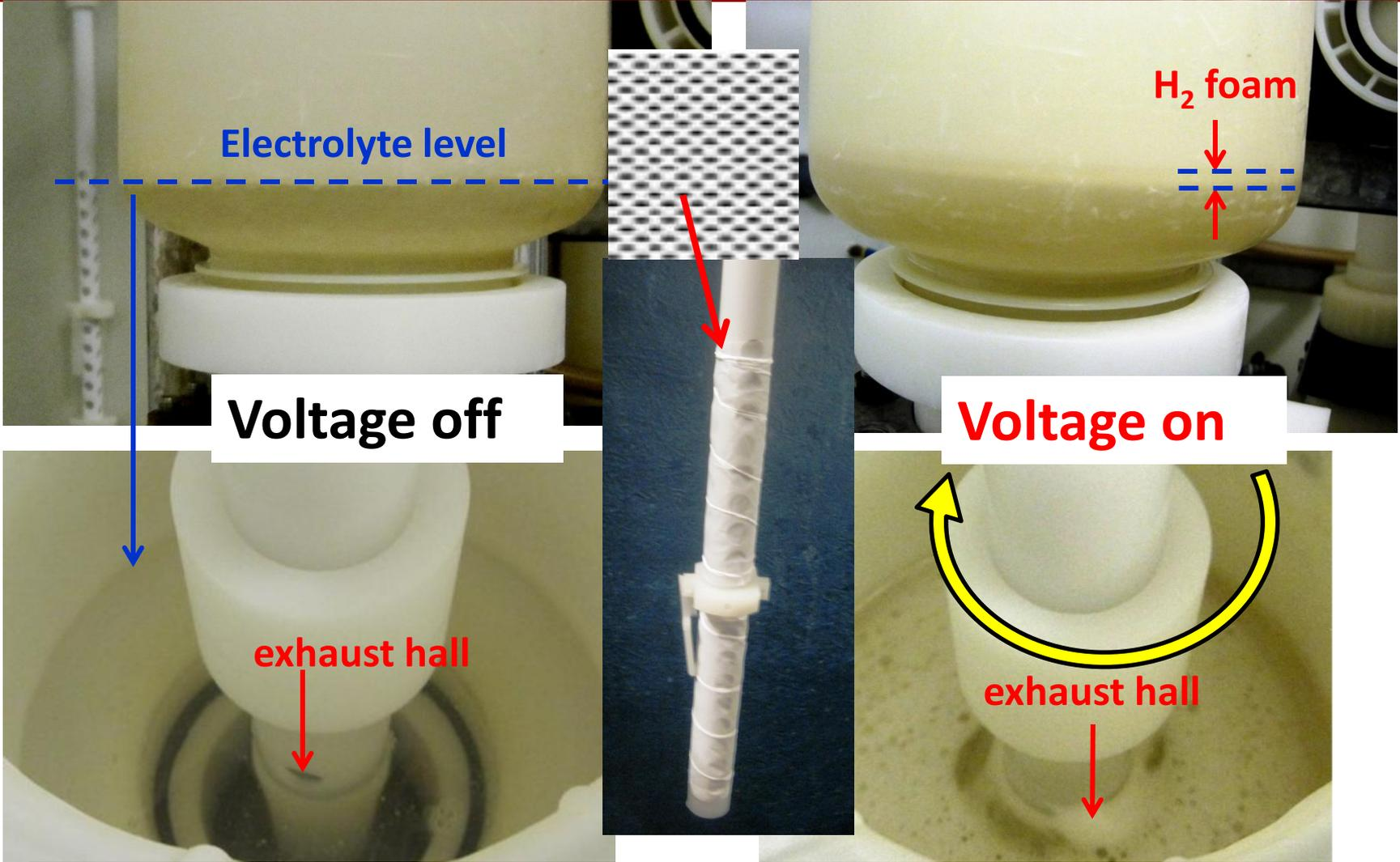
Cathode bag successfully guided hydrogen and reduced hydrogen foam layer.
