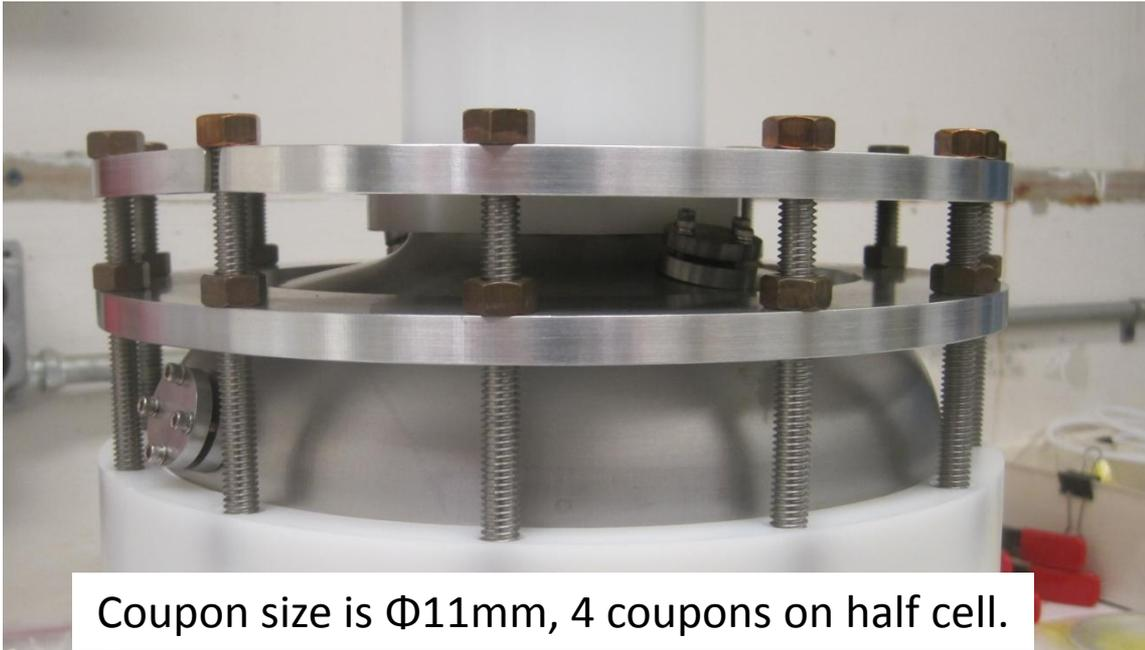
Coupon size is  $\Phi 11\text{mm}$ , 4 coupons on half cell.
