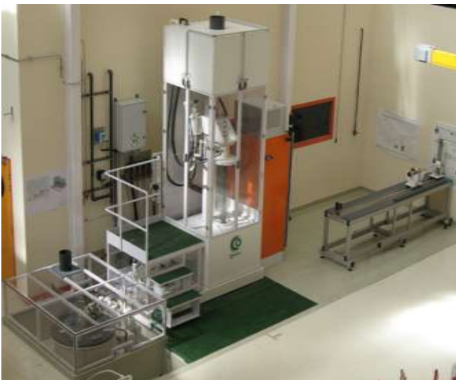
Operating Vertical EP station at Saclay: (Eucard beta=1 cavity, ESS HB ellipsicals, tested on 1.3 GHz single cells, 9-cells)
