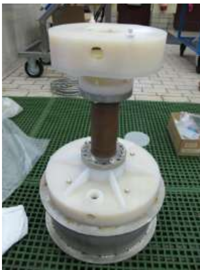
Vertical EP at CERN: First tests on a b=0.65 single cell cavity (S. Calatroni )
