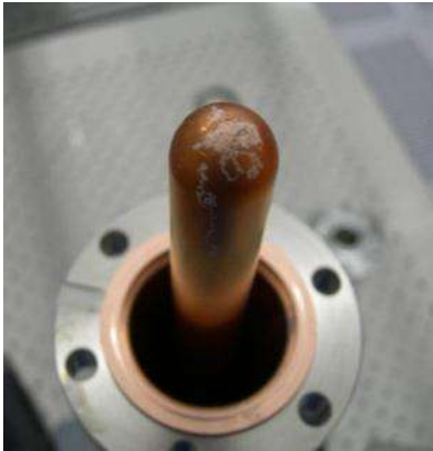
Discharge marks on coupler tip after high beta CM test (2010) Cavity Eacc limitation in CM = \frac{1}{2} max. Eacc in VT
